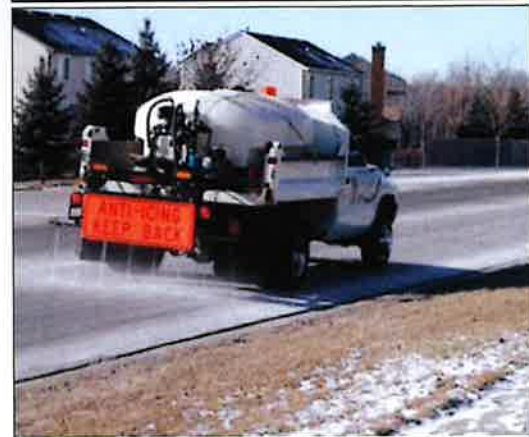
Typical anti-icing equipment for roadways.
