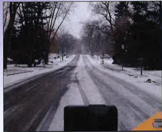
Anti-icing in left lane. No application in right lane.
