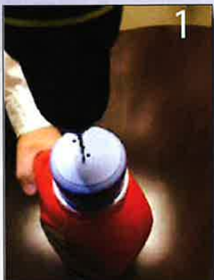
1 Drill eight to ten 1/8" holes into the top of the cap on whatever container you choose.
