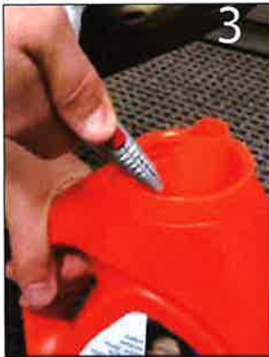
3 If there is an inner pour spout, carefully cut it out with razor knife.
