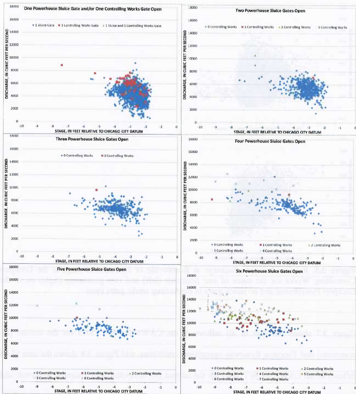
Figure 3.6. Relation between flow at Romeoville or Lemont and stage at the Lockport Controlling Works for the cases of one generator on at the Lockport Powerhouse and various numbers of powerhouse sluice gates and/or controlling works gates open.
