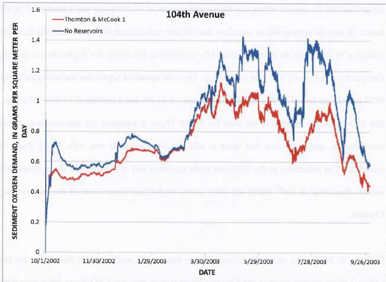
Figure 5.10. Sediment oxygen demand rates at 104 th Avenue on the Calumet-Sag Channel computed for the hydrologic conditions of Water Year 2003 for the cases of current inflows (No Reservoirs) and the Thornton and McCook Stage 1 reservoirs operational.
