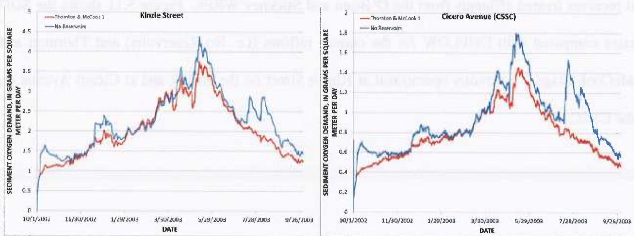
Figure 5.11. Sediment oxygen demand rates at Kinzle Street on the North Branch Chicago River and Cicero Avenue on the Chicago Sanitary and Ship Canal computed for the hydrologic conditions of Water Year 2003 for the cases of current inflows (No Reservoirs) and the Thornton and McCook Stage 1 reservoirs operational.
