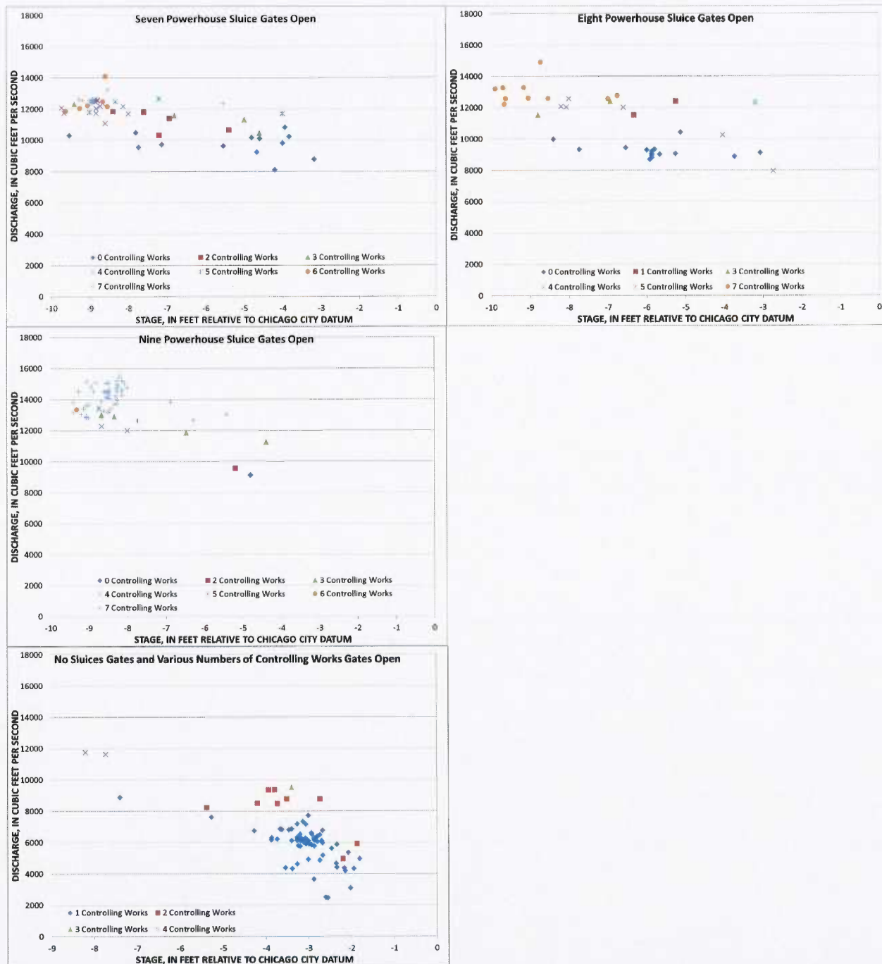
Figure 3.6. (cont.) Relation between flow at Romeoville or Lemont and stage at the Lockport Controlling Works for the cases of one generator on at the Lockport Powerhouse and various numbers of powerhouse sluice gates and/or controlling works gates open.
