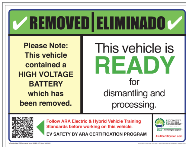
Figure 8: ARA high-voltage “battery removed” sticker. Source: ARA, 2020. 28
