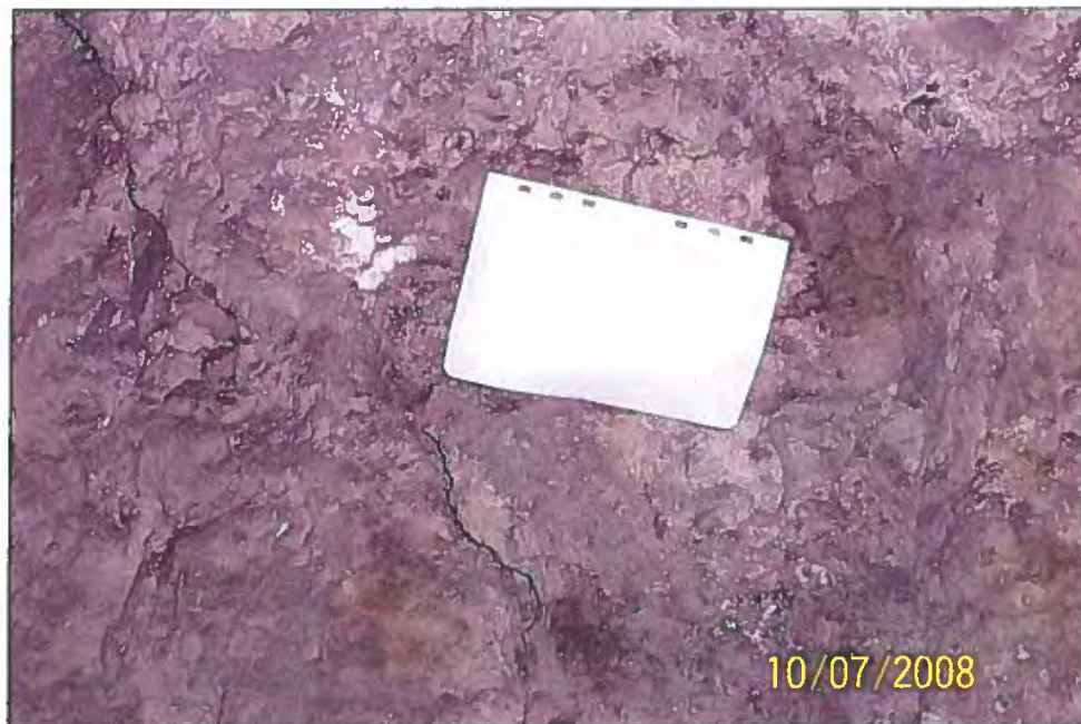
Figure 3-1. Example of Shear Zone Containing Calcite and Sulfide Mineralization
