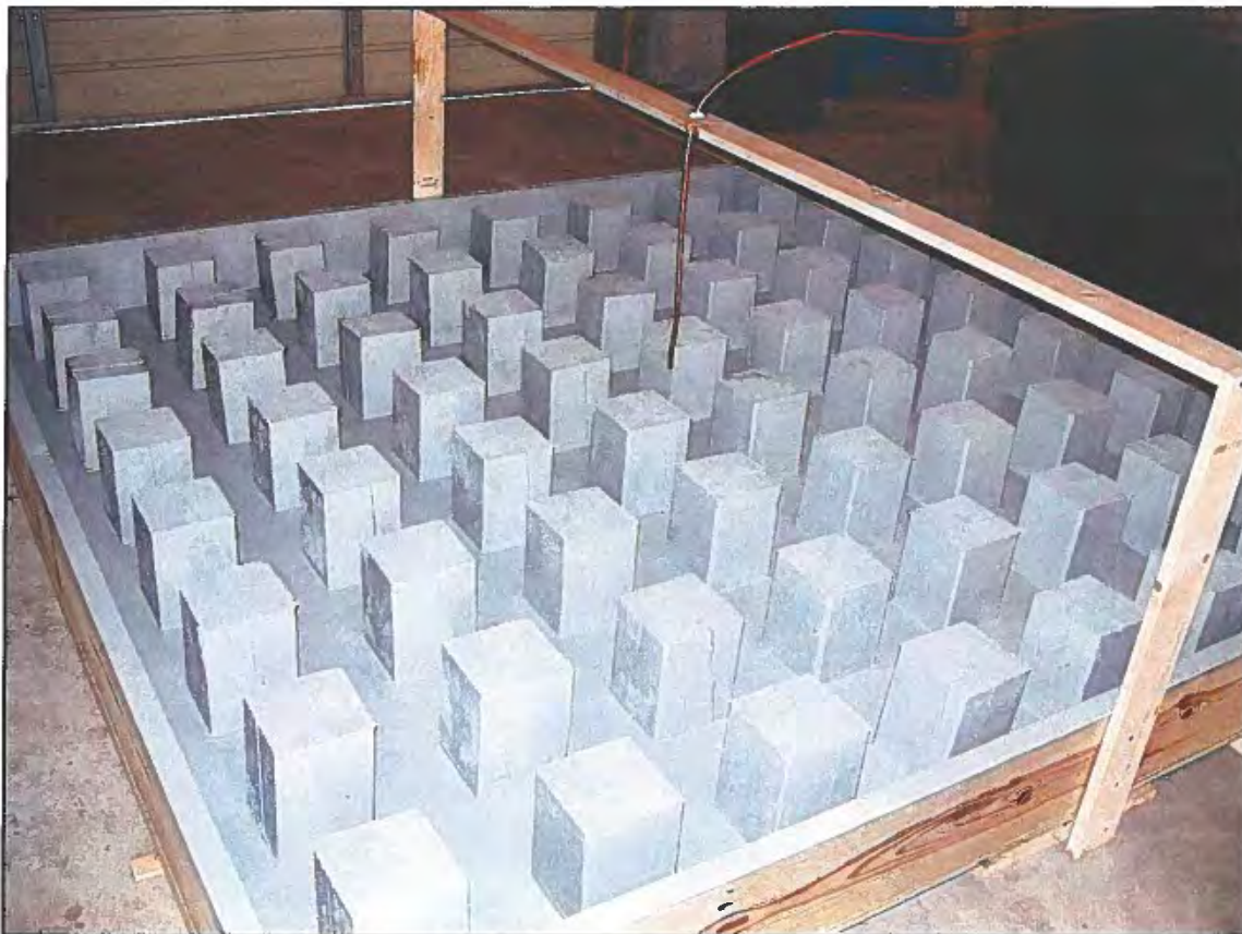
Photograph 13.1 - Scaled model of mine for simulation of lime sludge deposition
