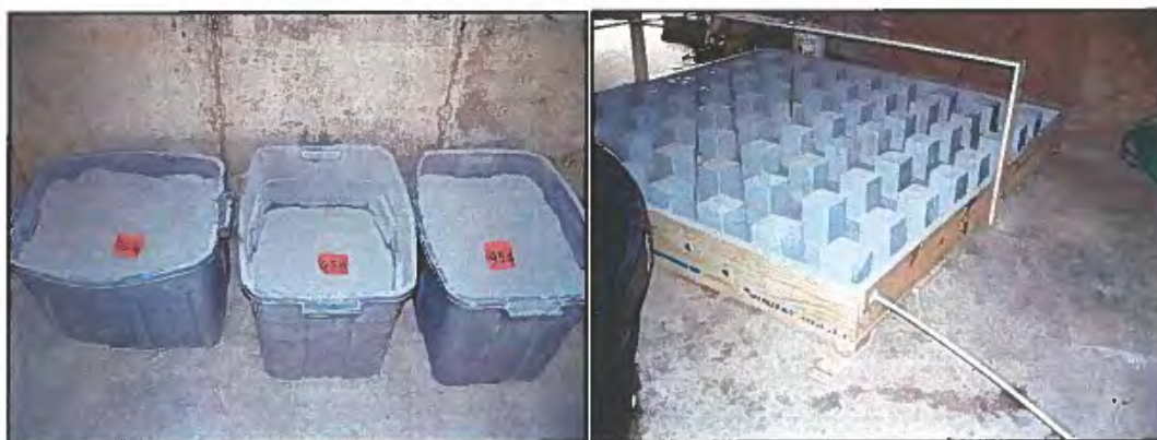
Photographs 13.4 and 13.5 - Dried and weighed lime powder and scaled model discharge line
