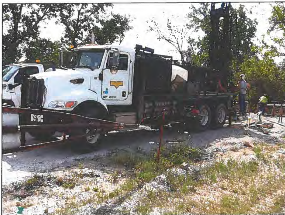
Photograph 5.1 – CME-75 Drill rig used for drilling and coring
