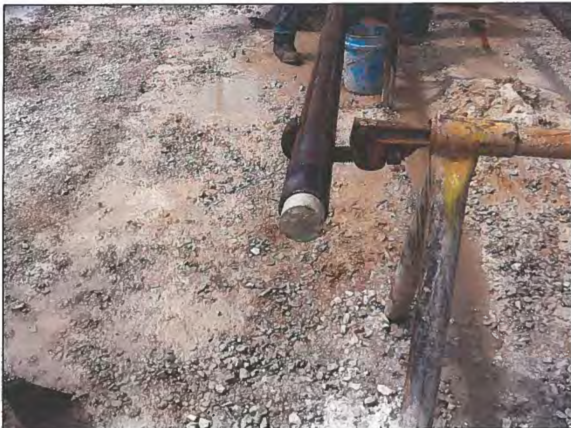
Photograph 5.4 – Rock core prior to retrieval from core barrel
