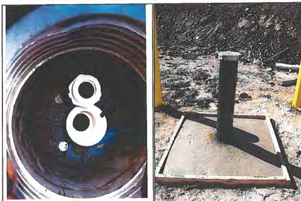
Photographs 7.15 and 7.16- Wellhead and GW sampling port (right)
