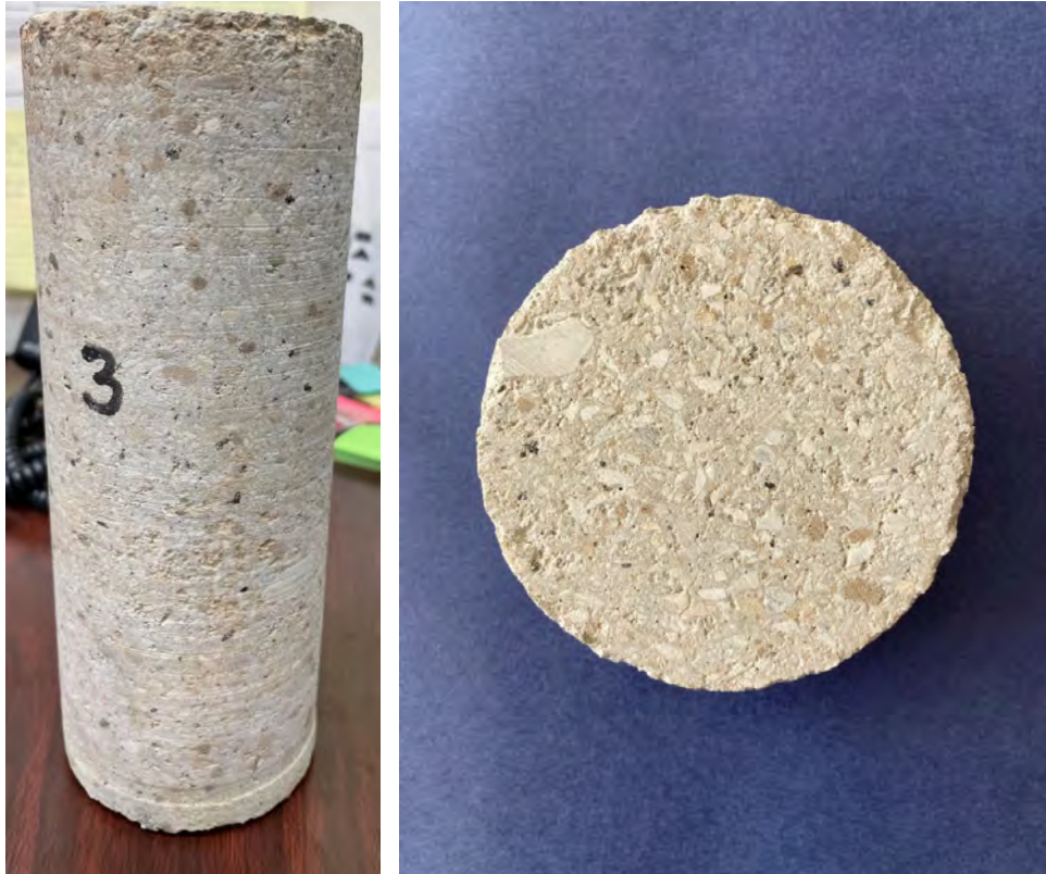
Figure 1. 3-inch diameter Poz-o-pac core sample reportedly extracted from the ash pond liner at Will County Generation Station. Photograph on the left and sample on the right provided by Ms. Kristen Laughridge Gale.
