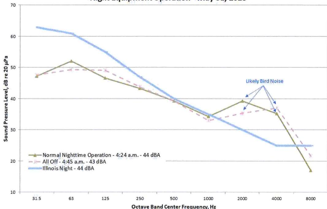
In order to investigate noise from equipment operating during the day, building personnel manually started rooftop mechanical equipment. Readings were taken during the early morning hours in order to minimize transportation noise, which would have made assessment of mechanical noise difficult or impossible during daytime hours.
