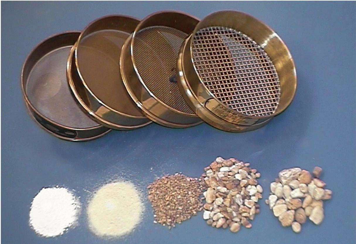
**Figure 2-2. Example of laboratory sieves for mechanical analysis for grain size distributions.** Shown (right to left) are sieve nos. 3/8-in (9.5-mm), No. 10 (2.0-mm), No. 40 (0.425 mm) and No. 200 (0.075 mm). Example soil particle sizes shown at the bottom of the photo include (right to left): medium gravel, fine gravel, medium-coarse sand, silt, and clay (kaolin) (FHWA, 2002b).
