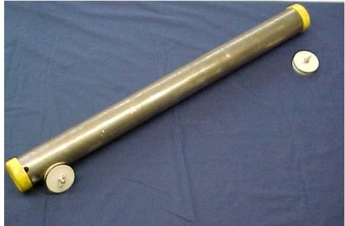
**Figure 3-9. Schematic of thin-walled (Shelby) tube (after ASTM D 4700) and photo of tube with end caps (FHWA, 2002b).**
