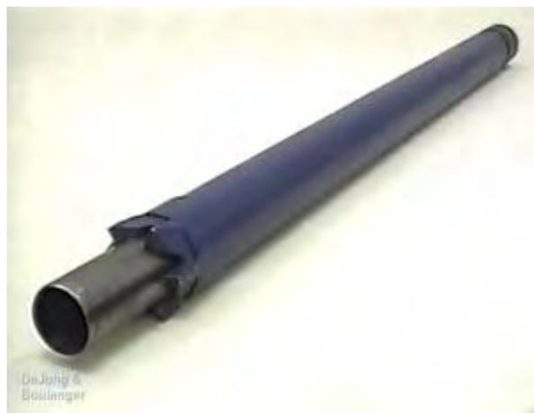
**Figure 3-12. Pitcher sampler (FHWA, 1997, 2002b).**
