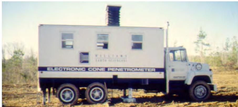
**Figure 3-29. Cone penetration testing from cone truck.**
