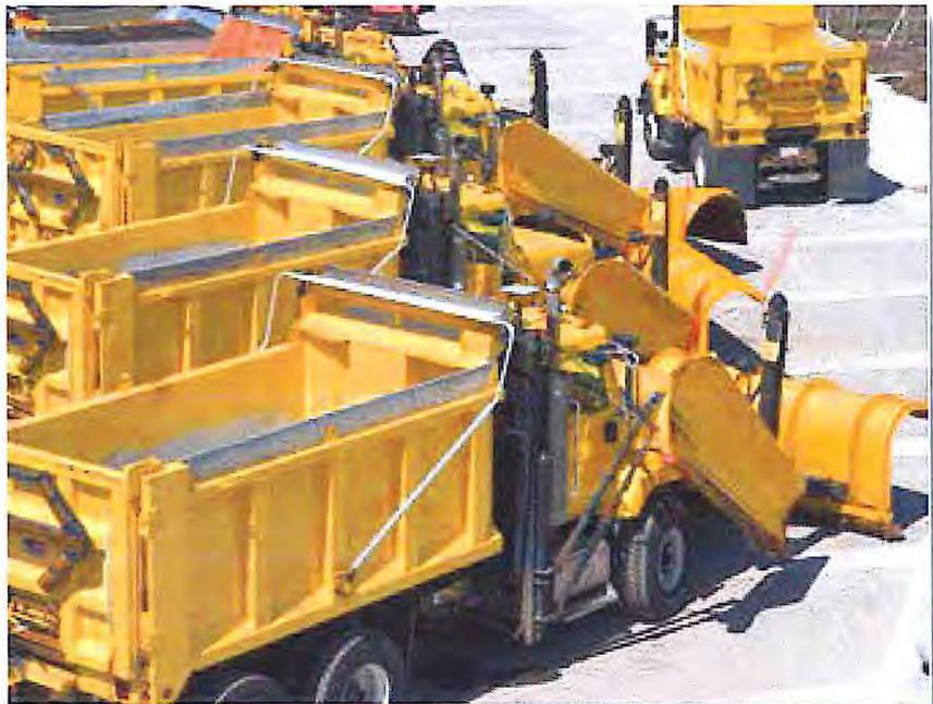
(Right-hand plows wear most rapidly on the left side, while the opposite is true for left-hand plows. Reversible plows may show wear on either side, depending upon operating time in each position.)
