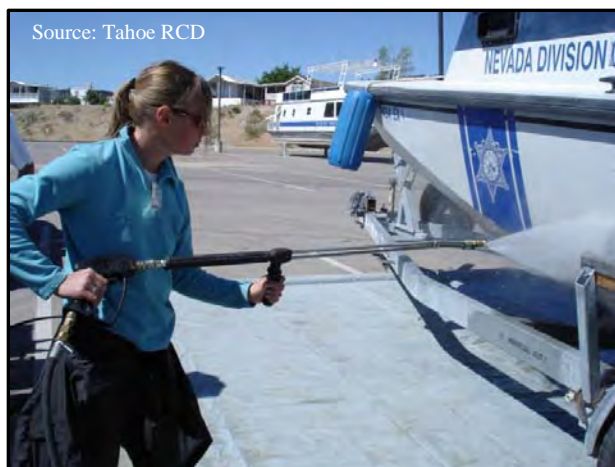
An employee of the Lake Tahoe Resource Conservation District uses a high pressure hot water nozzle to remove adult mussels from the hull of a boat.
