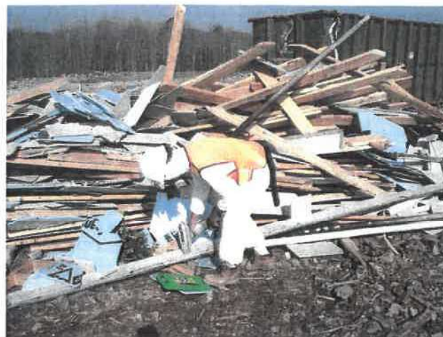
Fig. 3. Certified lead abatement worker XRF testing a painted surface during waste characterization study
