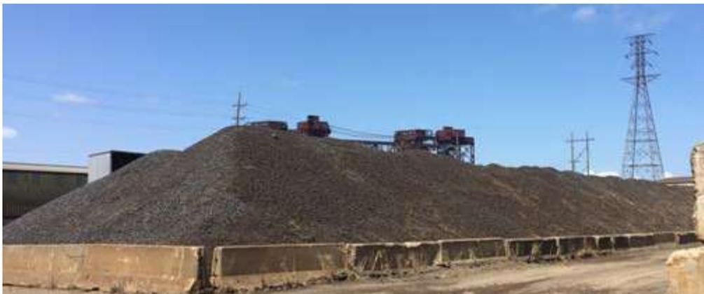
**Image 14 - Aggregate Pile - Pebble sizes range from 0.25 to 1.5 inches**
