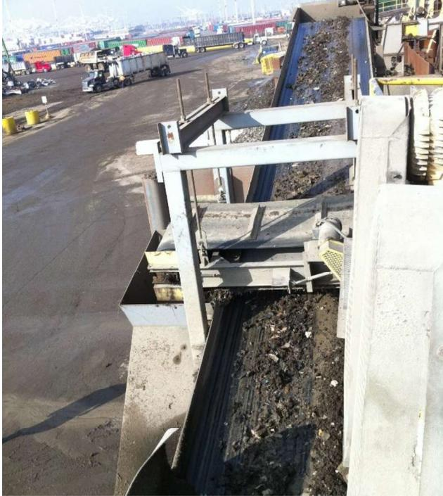
Chemically treated metal shredder residue is passed under a final magnet for recovery of ferrous metal at Schnitzer Steel, Inc., in Oakland.
