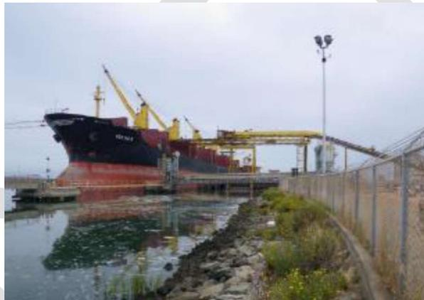
Loading sorted and shredded ferrous metals onto ship via conveyor system, Sims Metal Management, Redwood City, CA.
