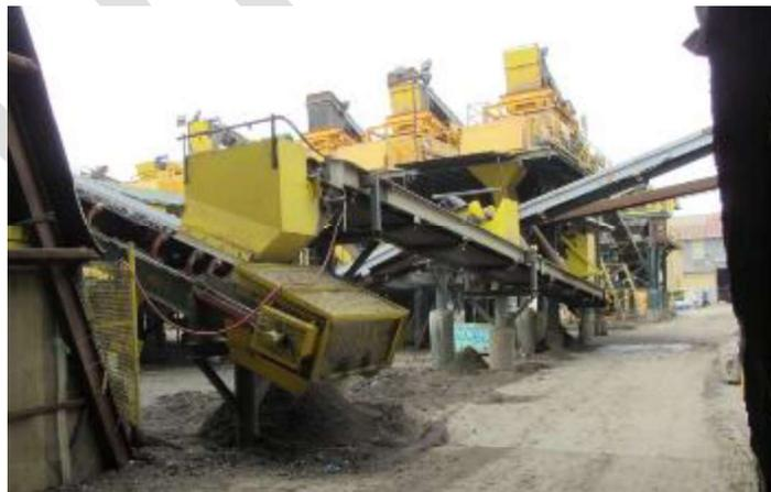
Conveyor belt lines used to transport material through the joint products plant and to the chemical treatment system at Schnitzer Steel, Inc., Oakland, CA.
