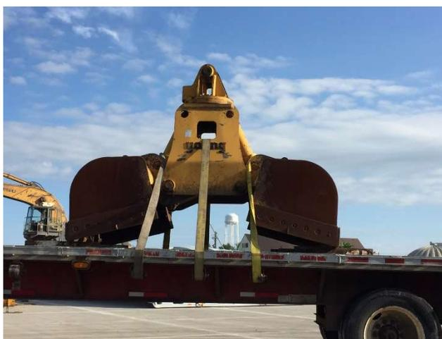
**Image 18 - Clamshell excavator attachment**
