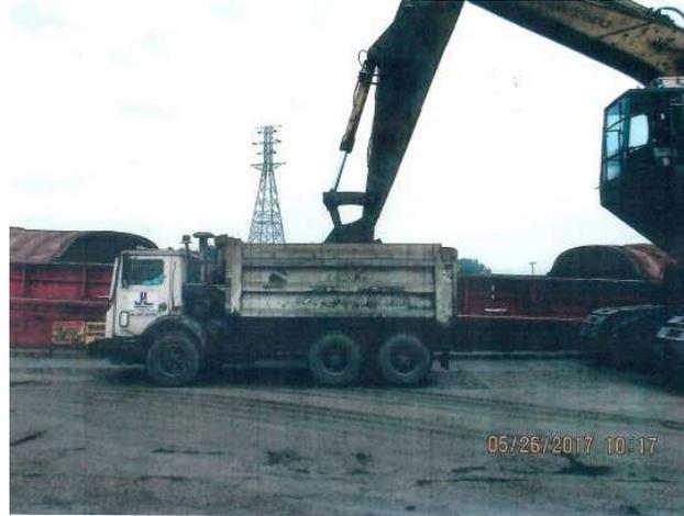
Image 7 - Excavator loading truck (note minimized "drop height")
