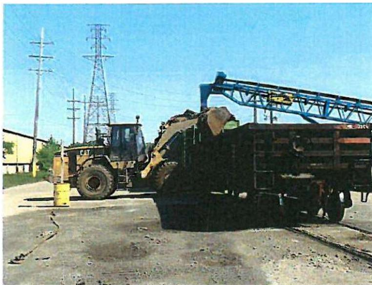
**Image 8 - Loading an open gondola car with pig iron. Note the front-end loader is operating on a concrete pad and no fugitive dust is present. The pig iron was sprayed with water prior to handling.**
