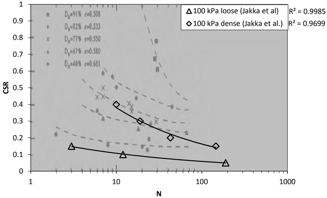
**Figure 22:** Plot of CSR versus number of loading cycles to liquefaction for surface impounded CCRs tested by Jakka et al (2010) at a confining pressure of 100 kPa. For comparison, curves for C778 sand at the same confining pressure are superimposed (Carraro et al 2003).
