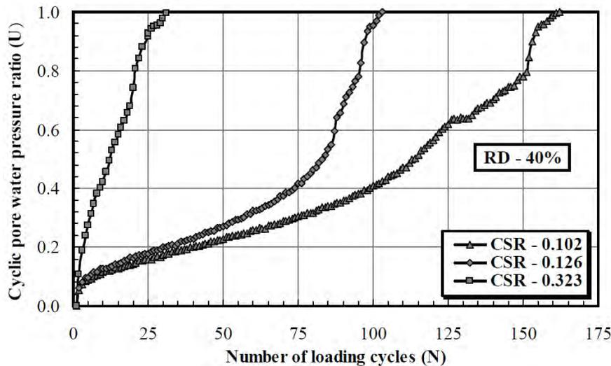
**Figure 19:** Plot of excess pore pressure ratio versus number of loading cycles for compacted Indian surface impoundment ash at different cyclic stress ratios and 1 Hz loading frequency (Mohanty et al. 2010).
