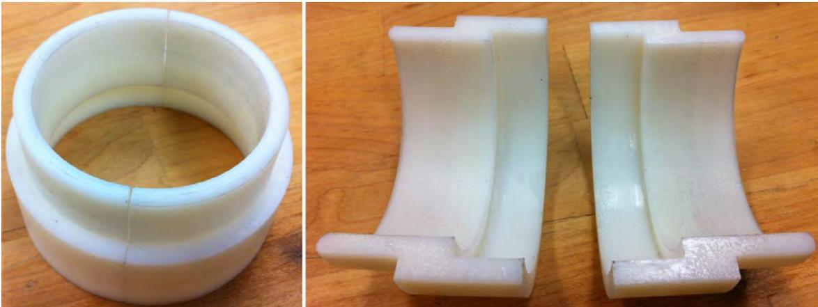
**Figure 37:** A custom-made split-collar to accommodate the additional volume of soil when the slurry is first placed in the specimen split-mold. This collar was machined out of nylon to fit the dimensions of the split-mold being used and the flexible collar used to accommodate the extra water volume when the slurry was placed.
