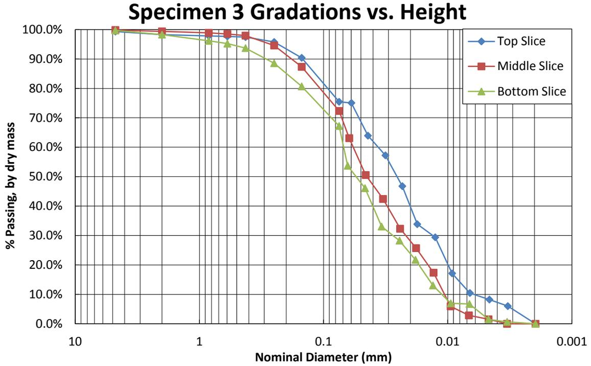
Figure 47: Plot comparing grain-size distribution across the height of specimen three.
