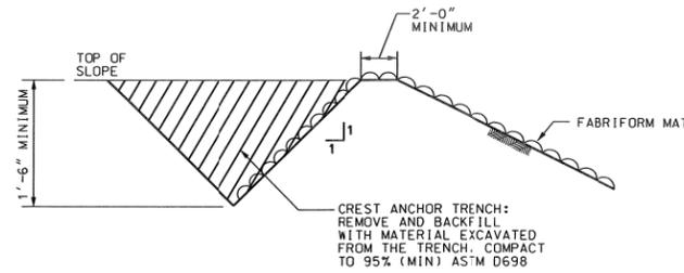
ANCHORAGE IF PROTECTION IS PROVIDED TO THE TOP OF THE SLOPE
