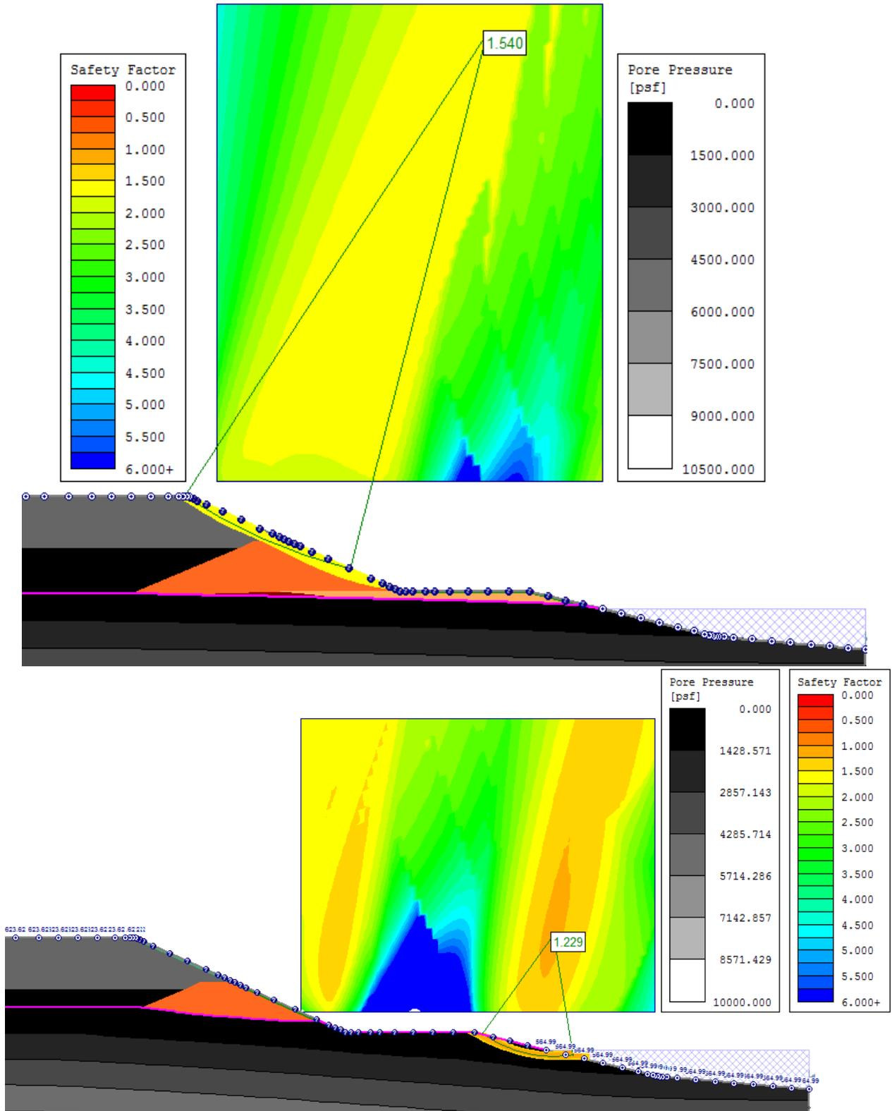
**Figure 30:** Analyses for an added upstream dry-disposed cell over the surface impoundment, for the in-situ water table (above) and for a hypothetical higher groundwater table (below). Slip surfaces with factors of safety between 1.5 and 1.6 are shown in the above case and between 1.2 and 1.3 for the below case.
