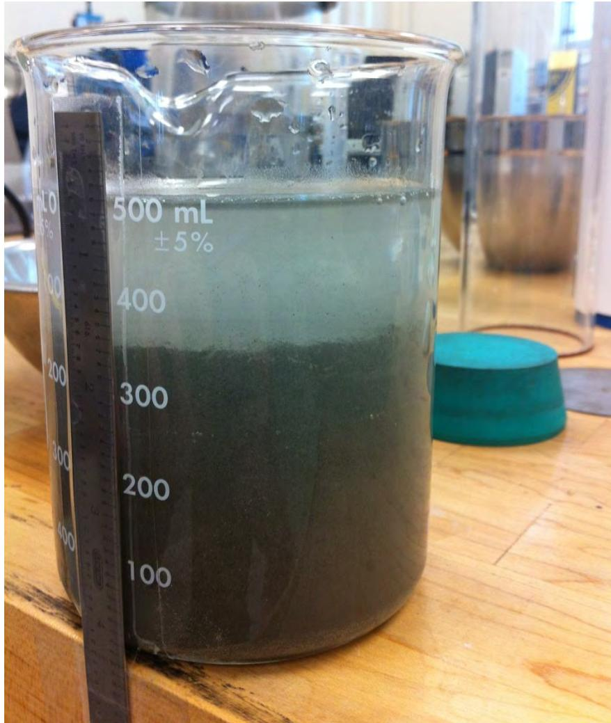
**Figure 44:** Each specimen slice volume was determined using water displacement. A 500 mL capacity beaker and a ruler incremented at 1/100" were used to do this. The vertical distance between a 100 mL addition of water to the beaker and the equation for the volume of a cylinder was used to calculate the diameter of the beaker; with the diameter known, it was determined that volumes could be measured accurately to  $\pm 1.4 \text{ cm}^3$ .
