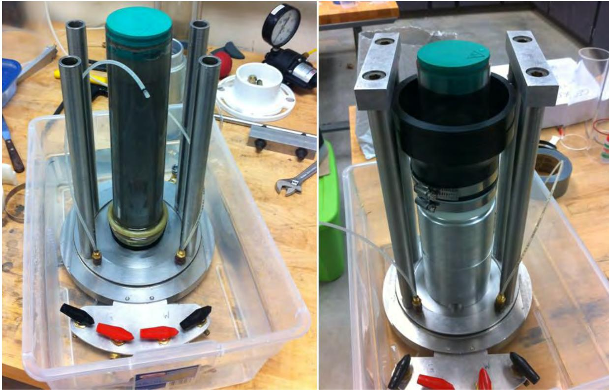
**Figure 40:** Rolling up the membrane around the mixing tube and placement of the specimen split-mold, the slurry extension collar, and the water extension collar after removal of the triaxial cell base from the water bath.
