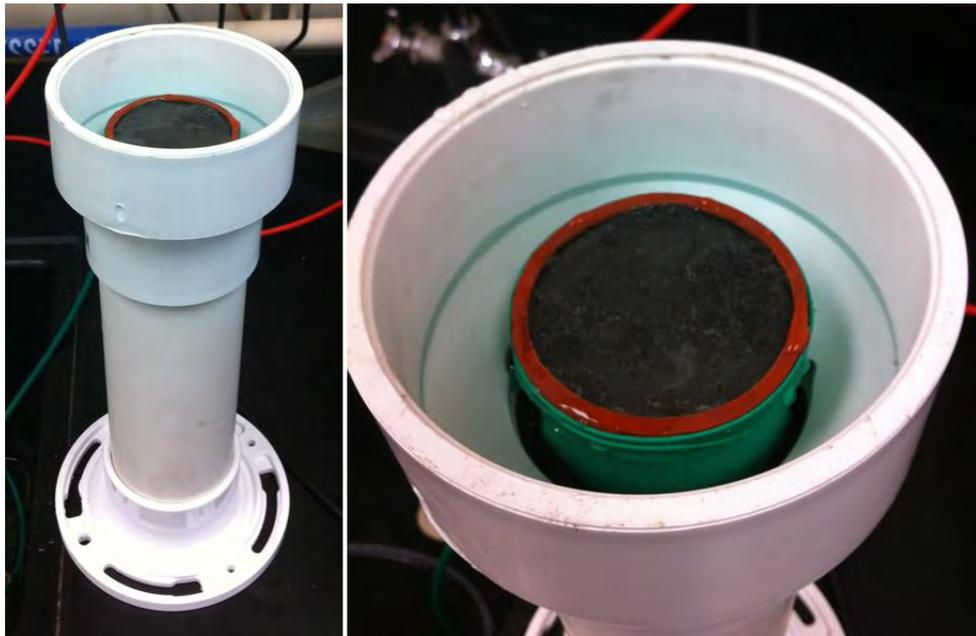
**Figure 35:** Water bath large enough to completely submerge the mixing tube and allow for easy placement of the porous disk and metal plate. The rubber membrane can also be seen rolled down around the mixing tube.
