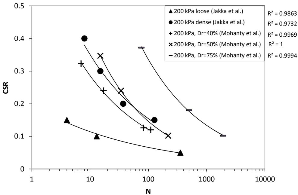
**Figure 23:** Plot of CSR versus number of loading cycles to liquefaction for different surface impounded CCRs tested by different researchers at 200 kPa confining stress. Jakka et al. loaded specimens at 0.1 Hz to 1 Hz and Mohanty et al. loaded specimens at 1 Hz.
