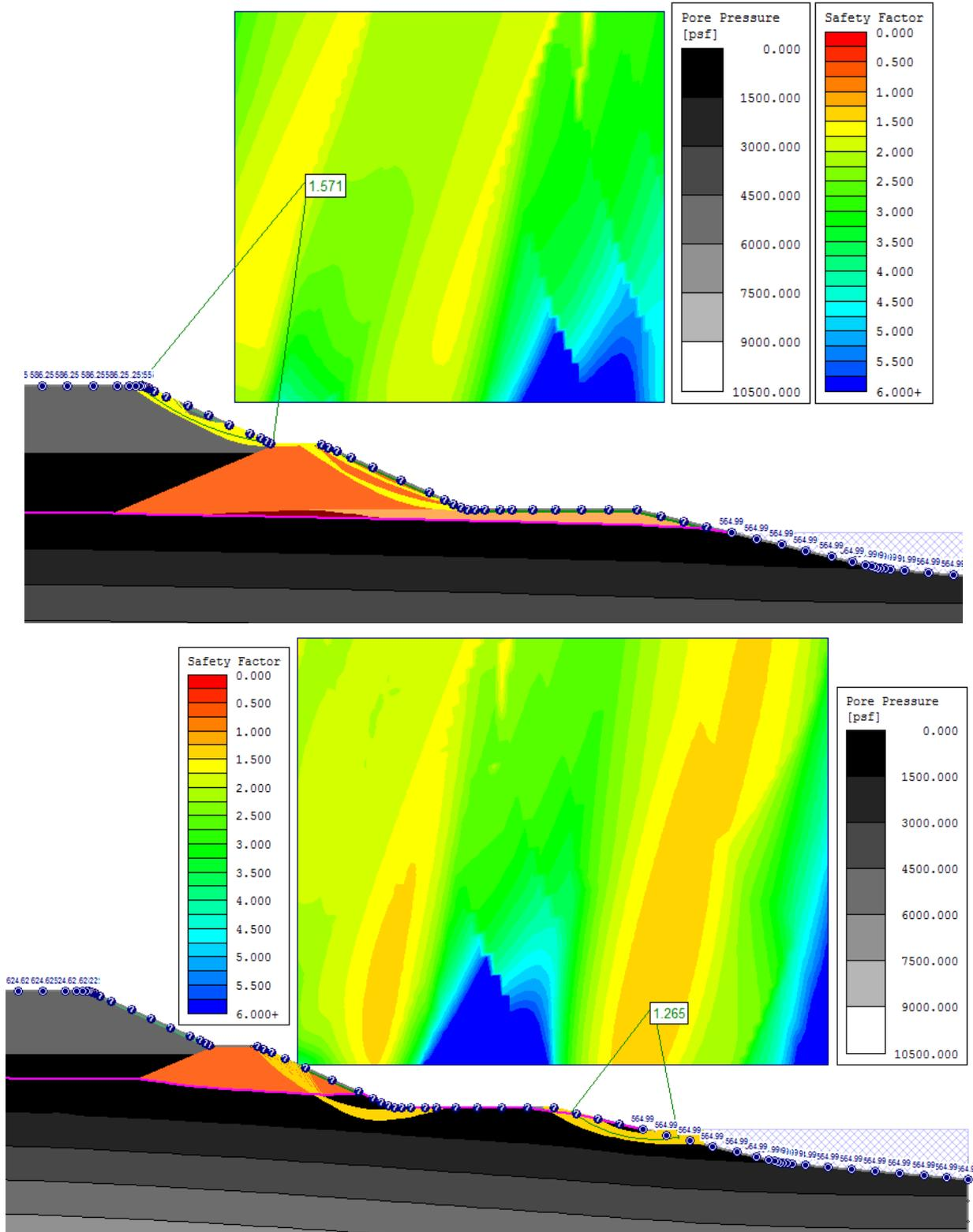
**Figure 31:** Analyses for an added upstream dry-disposed cell above the surface-impoundment for the in-situ groundwater table (above) and for a hypothetical higher groundwater table (below). Slip surfaces with factors of safety between 1.5 and 1.7 are shown for the above case and between 1.2 and 1.4 for the below case.
