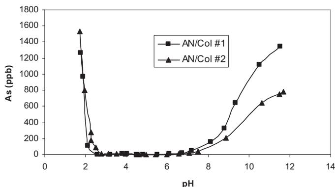
Figure 2. Basic leaching results for As from ash AN/Col #1 and AN/Col #2. Experimental conditions: S/L = 1:10; temperature = 20 – 25 °C; equilibration time = 24 hours.
