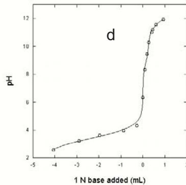
Figure 1 Titration and curve fitting results for washed ashes: (a) AN/Col #1; (b) AN/Col #2 (DI water washed); (c) AN/Col #2 (0.2M NaOH washed); and (d) AN/NRT #2. Ionic strength = 0.01 M (NaNO<sub>3</sub>), temperature = 20 – 25 °C; equilibration time = 24 hours.
