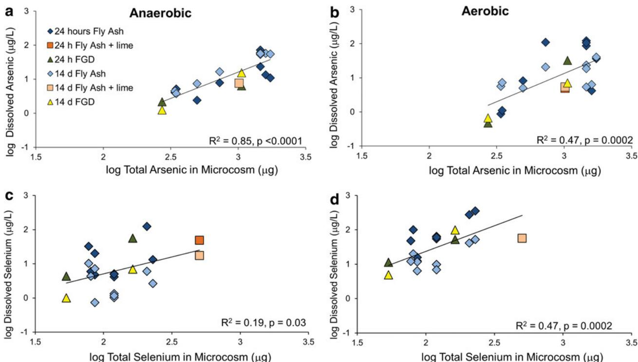
**FIG. 5.** Correlations between total element content in ash material and dissolved element content in sediment/ash slurry microcosms: (a) arsenic in anaerobic microcosms; (b) arsenic in aerobic microcosms; (c) selenium in anaerobic microcosms; and (d) selenium in aerobic microcosms. Each data point represents a single microcosm.
