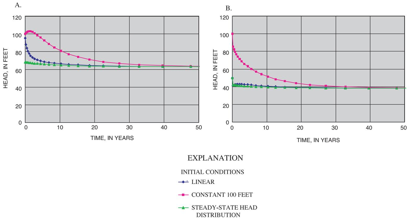
**Figure 15.** Head in a cell through time in response to a well discharging at a rate of 100,000 ft<sup>3</sup>/d: (A) the head in layer 1 at the divide, and (B) the head in the cell with the discharging well in layer 3.
