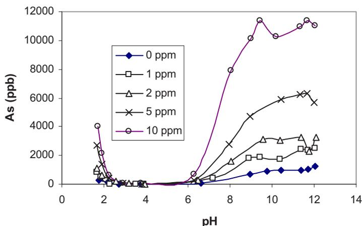
Figure 5. As(V) partitioning results for 0.2 M NaOH washed ash AN/Col #2. Experimental conditions: S/L = 1:10; ionic strength = 0.01M NaNO<sub>3</sub>; temperature = 20 – 25 °C; equilibration time = 24 hours.
