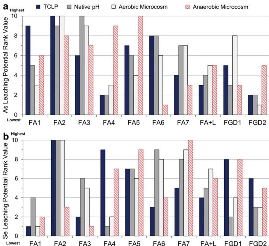
**FIG. 6.** Comparison of 10 coal ash samples tested in leaching studies (TCLP, DI water leaching, and sediment/ash microcosm tests). Ash samples were assigned integer values between 1 and 10 based on (a) leachable arsenic per g of ash; and (b) leachable selenium per g of ash at the 24 h time point for each leaching test.
