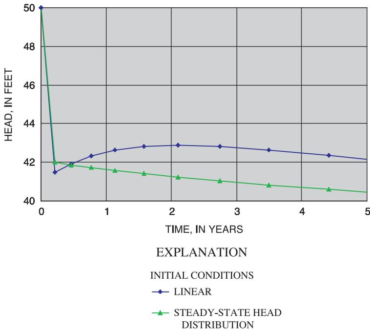
**Figure 16.** Head in the well for the first 5 years after the start of pumping for the cases using the initial conditions of the steady-state head distribution and the linearly varying head distribution.
