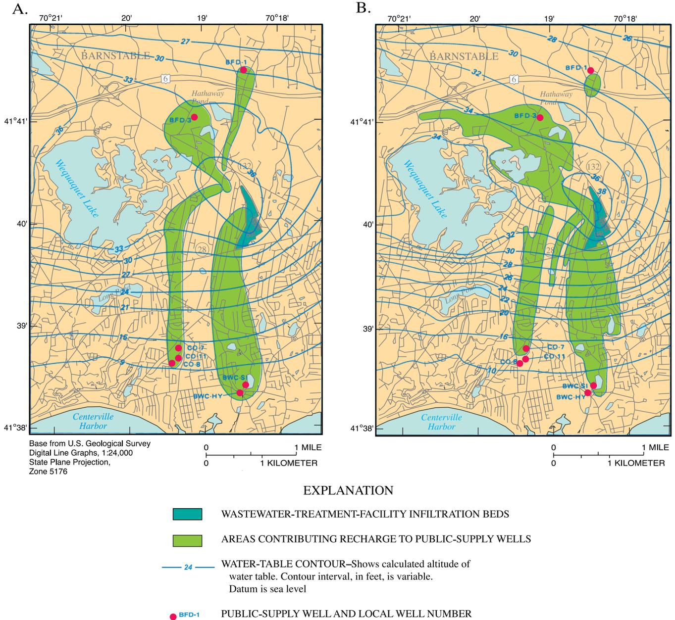
**Figure 9.** Comparison of areas contributing recharge to seven public-supply wells as determined by two different numerical models, Cape Cod, Massachusetts: (A) results from a two-dimensional single-layer model, and (B) results from a three-dimensional eight-layer model. (Modified from Barlow, 1994; and Franke and others, 1998.)
