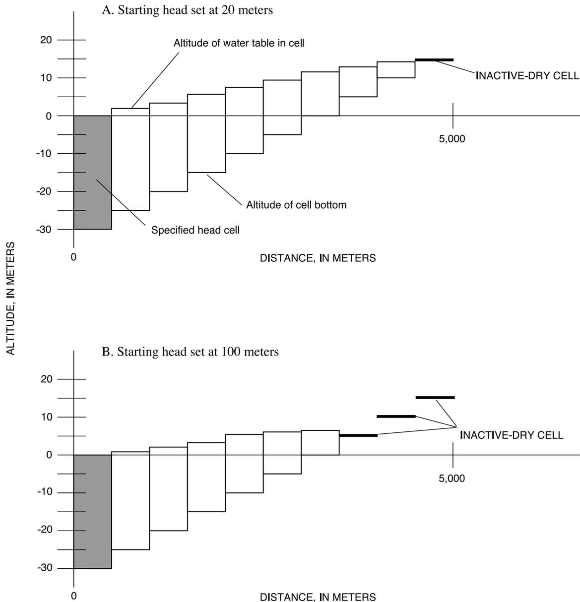
**Figure 17.** Cross-sectional view of a finite-difference representation simulating a variable thickness ground-water system with flow to a specified head due to areal recharge: (A) starting head set at 20 meters, and (B) starting head set at 100 meters. (From Reilly, 2001.)
