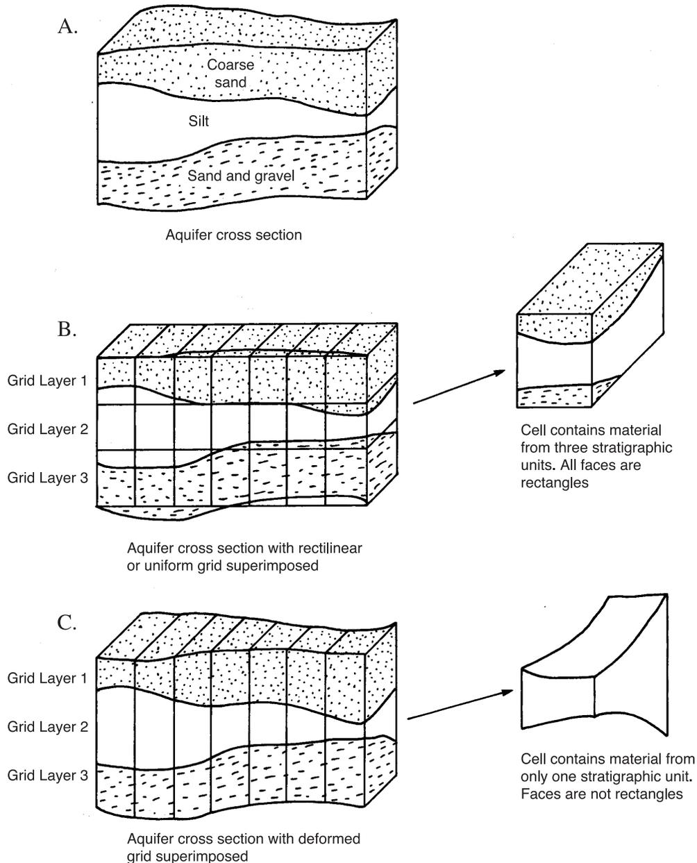
**Figure 6.** Schemes of vertical discretization for (A) aquifer cross section, (B) aquifer cross section with rectilinear or uniform grid superimposed, and (C) aquifer cross section with deformed grid superimposed.
