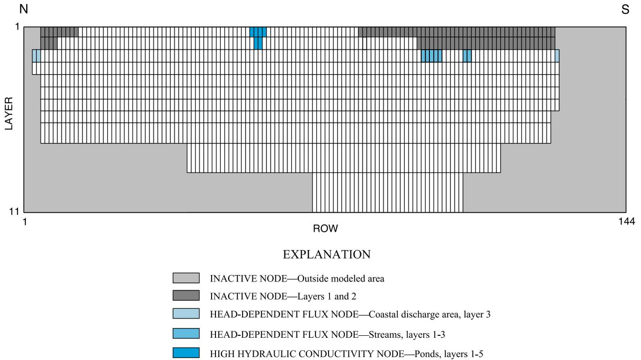
**Figure 7C.** Horizontal and vertical discretization using uniform layers for the model simulating ground-water flow on Cape Cod, Massachusetts. Vertical grid using uniform layers along column 85. (Modified from Masterson and others, 1997.)
