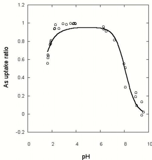
Figure 6. The adsorption results of As(V) onto washed ash AN/Col #2. Experimental conditions: metal concentrations = 1 - 10 mg/L; S/L = 1:10; ionic strength = 0.01M ( $\text{NaNO}_3$ ); temperature = 20 – 25 °C; equilibration time = 24 hours.
