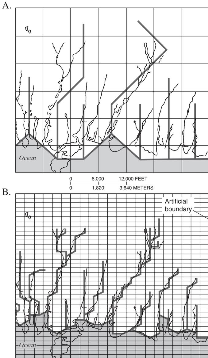
**Figure 2.** Representation of stream and shoreline boundaries on Long Island, New York, (A) as represented in a regional ground-water flow model grid, and (B) as represented in a sub-regional ground-water flow model grid. (Modified from Buxton and Reilly, 1987.)
