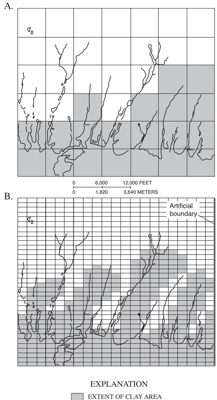
**Figure 1.** Extent of the south-shore confining unit on Long Island, New York, (A) as represented in a regional ground-water flow model grid, and (B) as represented in a sub-regional ground-water flow model grid. (Modified from Buxton and Reilly, 1987.)
