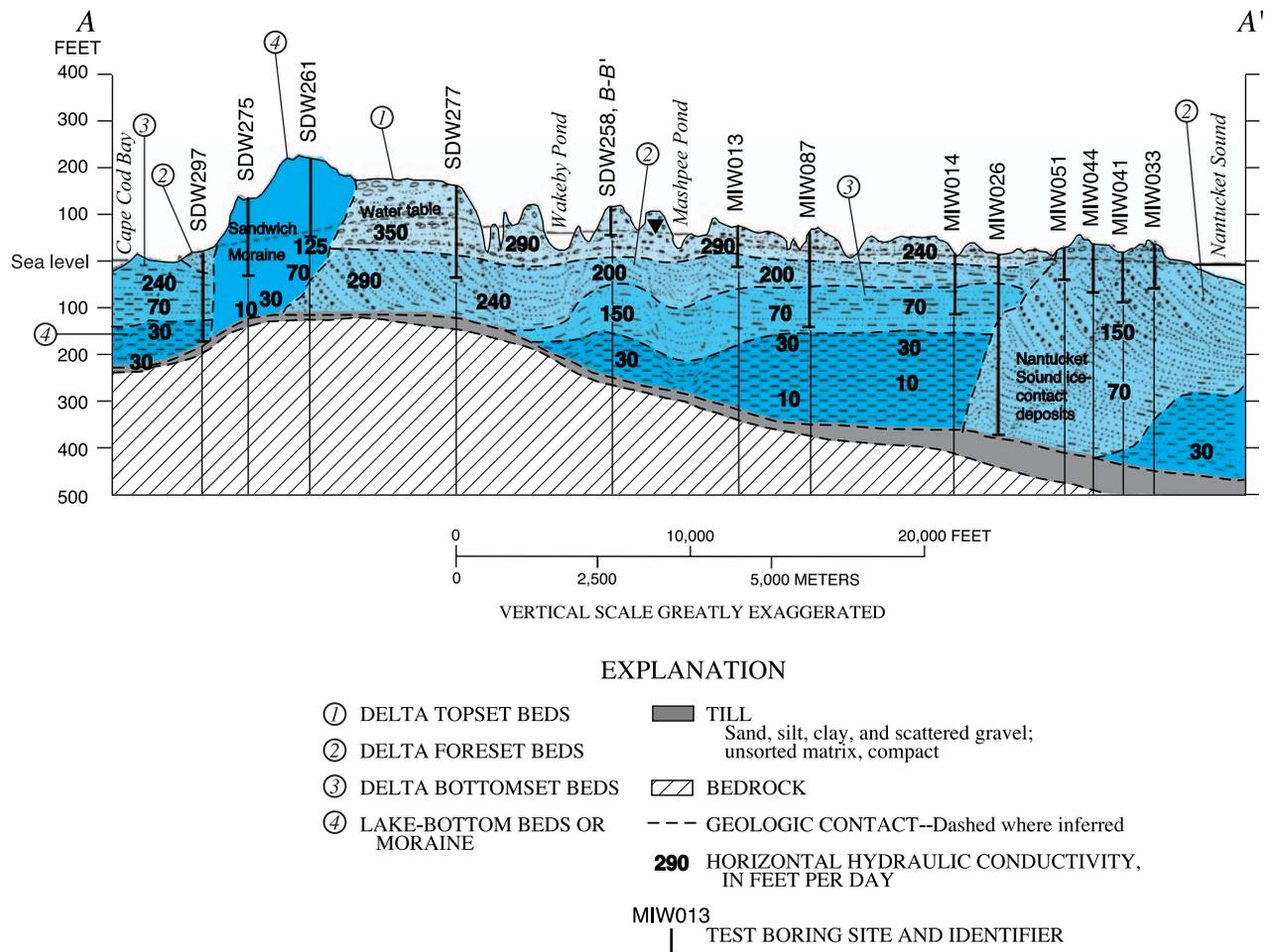
**Figure 7B.** Horizontal and vertical discretization using uniform layers for the model simulating ground-water flow on Cape Cod, Massachusetts. Hydrogeologic cross section near column 85. (Modified from Masterson and others, 1997.)
