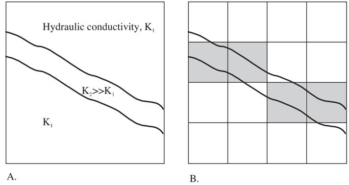
**Figure 4.** Large finite-difference cells may be inadequate to represent some important features of a ground-water system. (A) Map of the distribution of horizontal hydraulic conductivity showing a channel of high hydraulic conductivity. (B) Finite-difference cells representing the high hydraulic-conductivity channel are no longer continuous, because there is no direct connection between diagonal cells in the finite-difference method.
