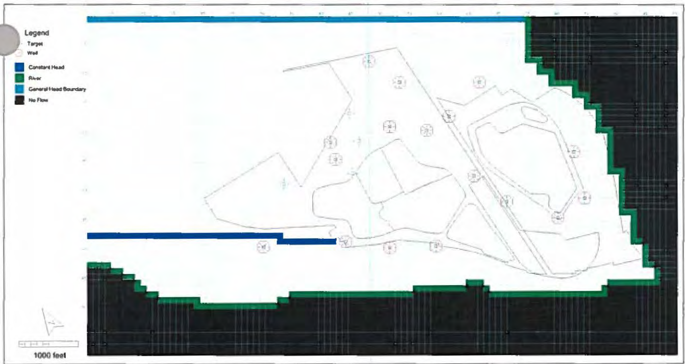
Figure 3-1. MODFLOW and MT3DMS Grid and Boundary Conditions for Layer 1 (top) and Layer 2 (bottom).
