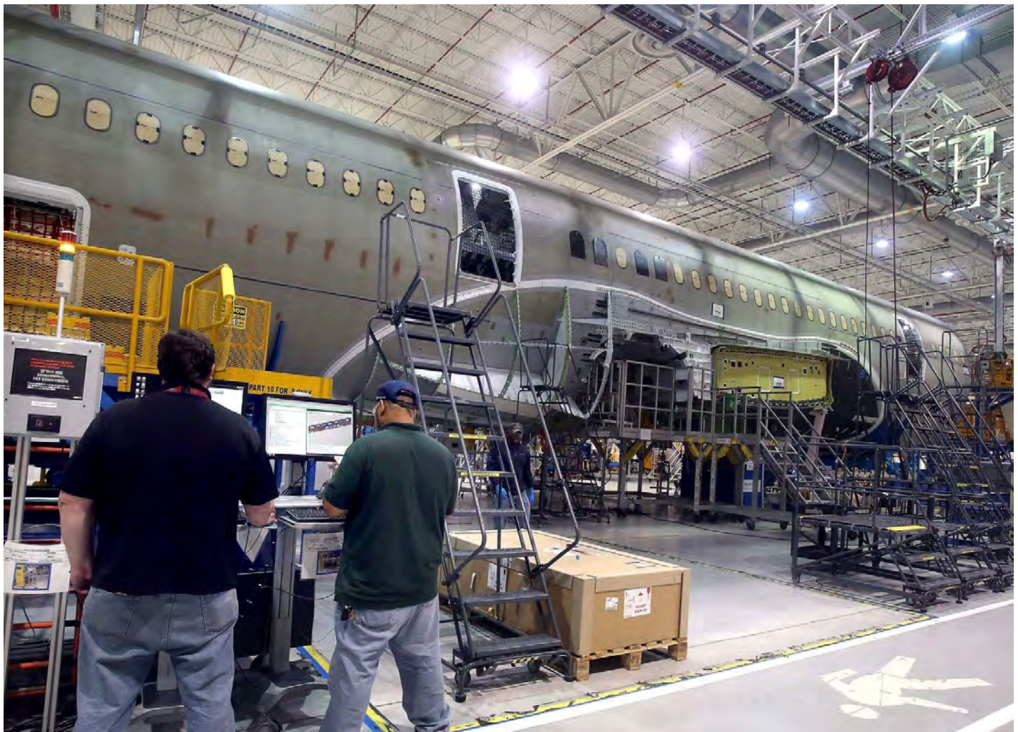
Boeing South Carolina workers put together the 787 Dreamliner midbody sections at the company's North Charleston campus.
