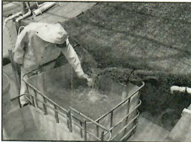
Bottle Grab Samples and Flow Rate Measurements Taken During Testing
