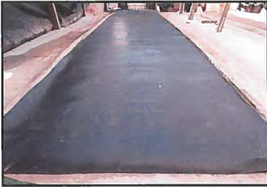
Test Slope Prepared and Liner Installed (Typical)
