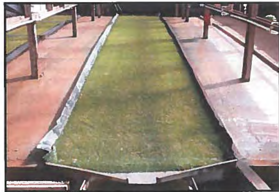
Sand/Cement Ballasted Slope - After Rainfall
