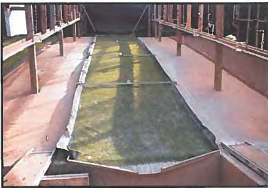
Slope Ready for Rainfall
