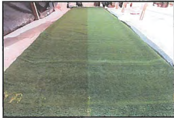
Test Slope Prepared and Liner Installed (Typical)
