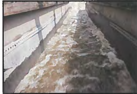
Highest Shear = Maximum Flow in 20% Flume
