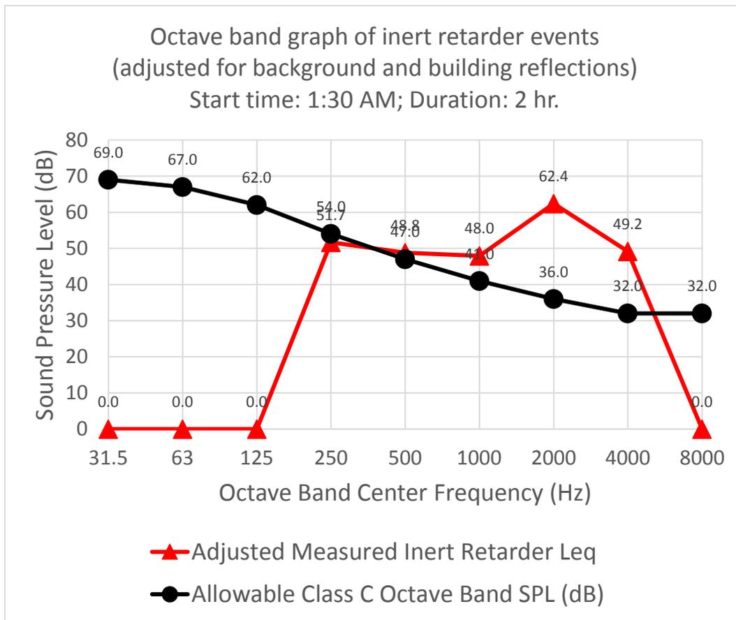
**Figure 4. Octave band sound pressure levels for adjusted measured inert retarder  $L_{eq}$  for Period 1, 1:30 AM to 3:30 AM, April 11, 2018, outside Hyatt Place hotel and allowable nighttime levels from Class C land emitted to Class A land.**
