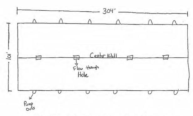
The Pit is 101' x 304' and is 8' deep. The Concrete is reinforced with rebor. There is a center support wall in the middle and 4 flow through at the bottom of the center wall. There are also 6 pumpouts (PTO driver Certificals) on each side of the Pit. The Floor is 100% total stats
