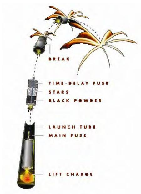
**Figure 3-1: Display Firework Schematic**
