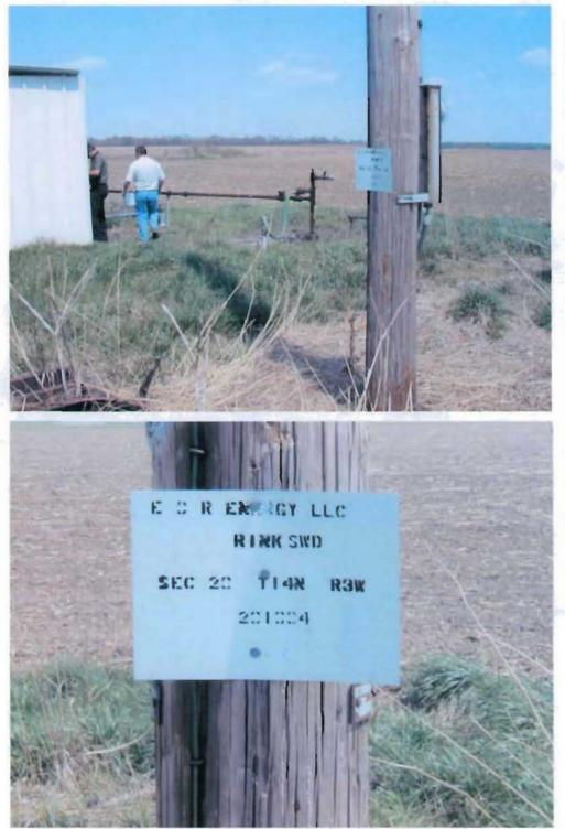
Date: 04/19/2005 Time: 1:11 pm **Direction: Northeast** Photo by: Rich Johnson Exposure #: 007 **Comments: Photo** shows Rink #1 salt water disposal well with gas injection located on the Rink Lease. Note the wellhead and associated pipes. The shed with an air compressor is located left (to the west) of the wellhead.
