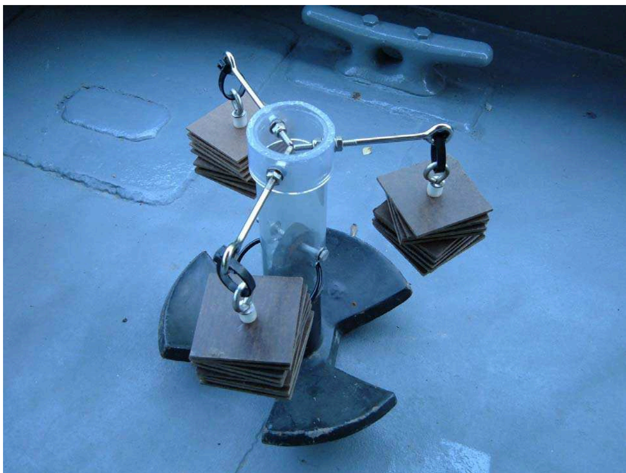
Figure 2. MWRDGC's Hester-Dendy Sampling Apparatus. Organisms are removed from the plates after the samplers are left in the CAWS for 7 to 14 weeks. (Photo courtesy of Mr. Thomas Minarik, MWRDGC)
