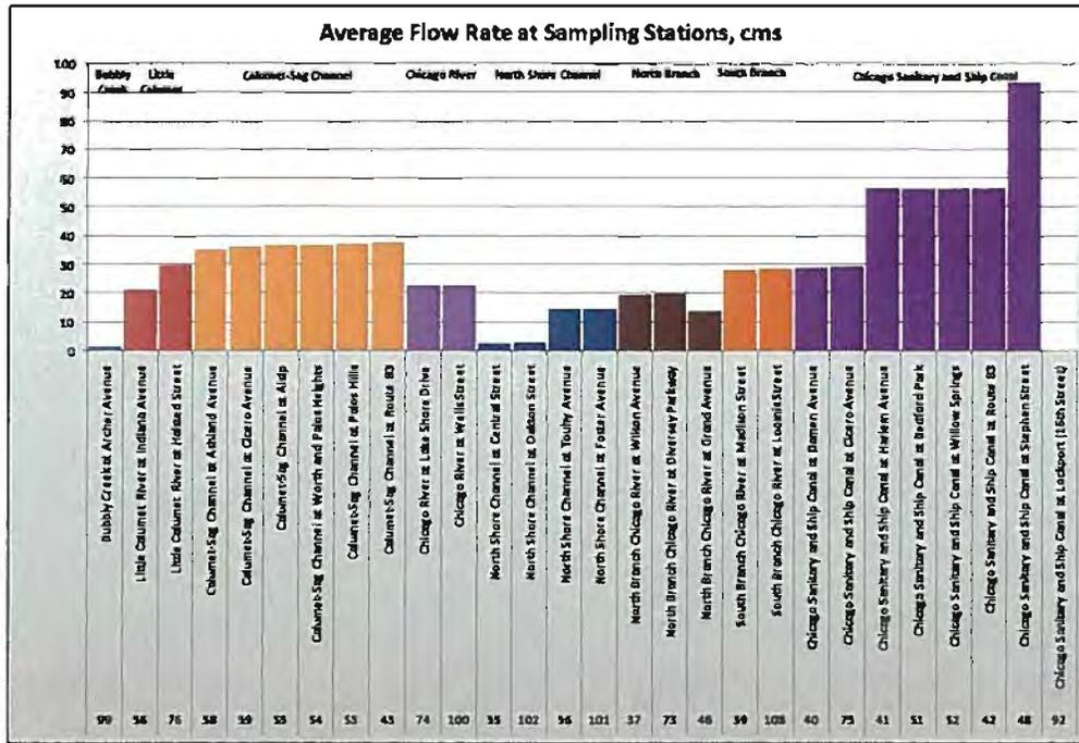
Figure 4-8: Average Flow Rate at CAWS Sampling Stations.
