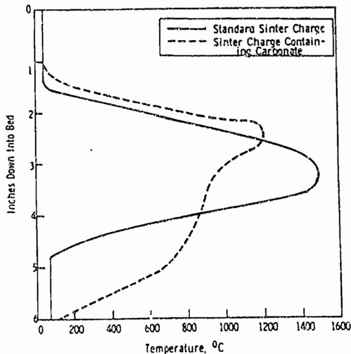
Fig. 2-9. Temperature Distribution for Two Sinter Mixes.
