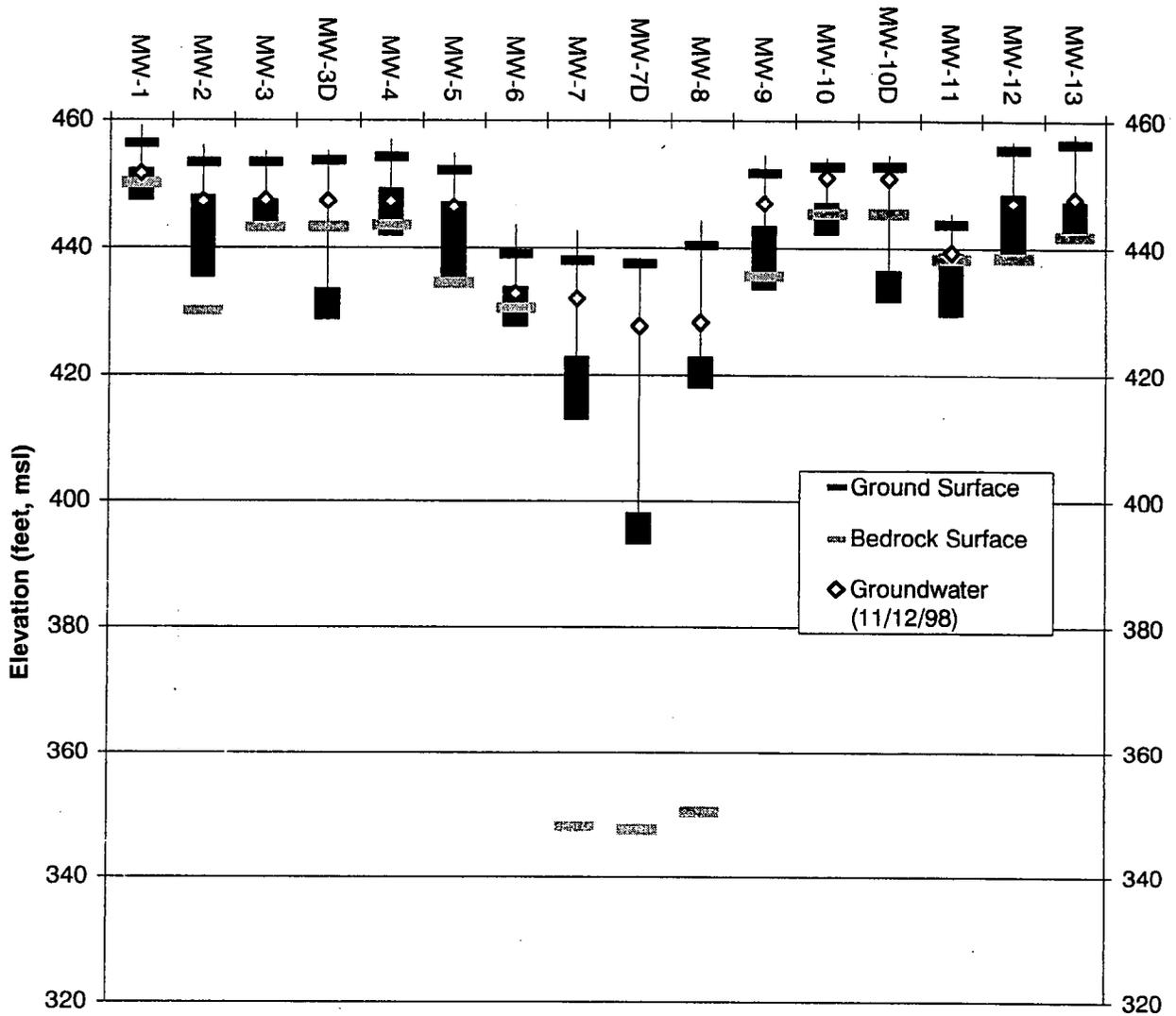
Figure 2. Elevation of well screens, ground surface, bedrock surface, and groundwater. Bedrock surface depths for MW-7, MW-7D, and MW-8 are estimated.
