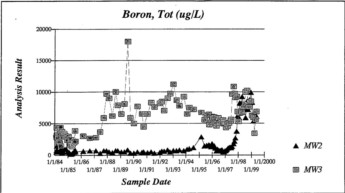
Figure 11. Historical boron concentrations at MW-2 and MW-3.
