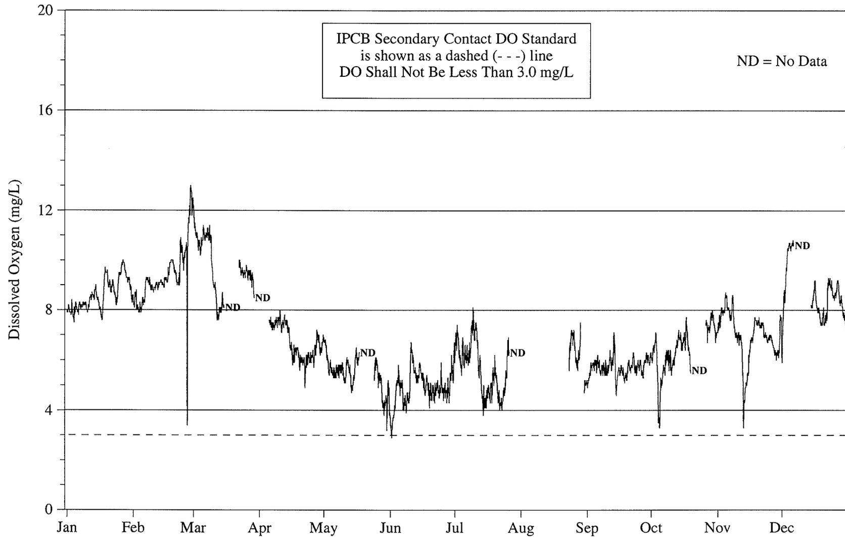
FIGURE 21: DISSOLVED OXYGEN CONCENTRATION MEASURED HOURLY AT ROUTE 83
