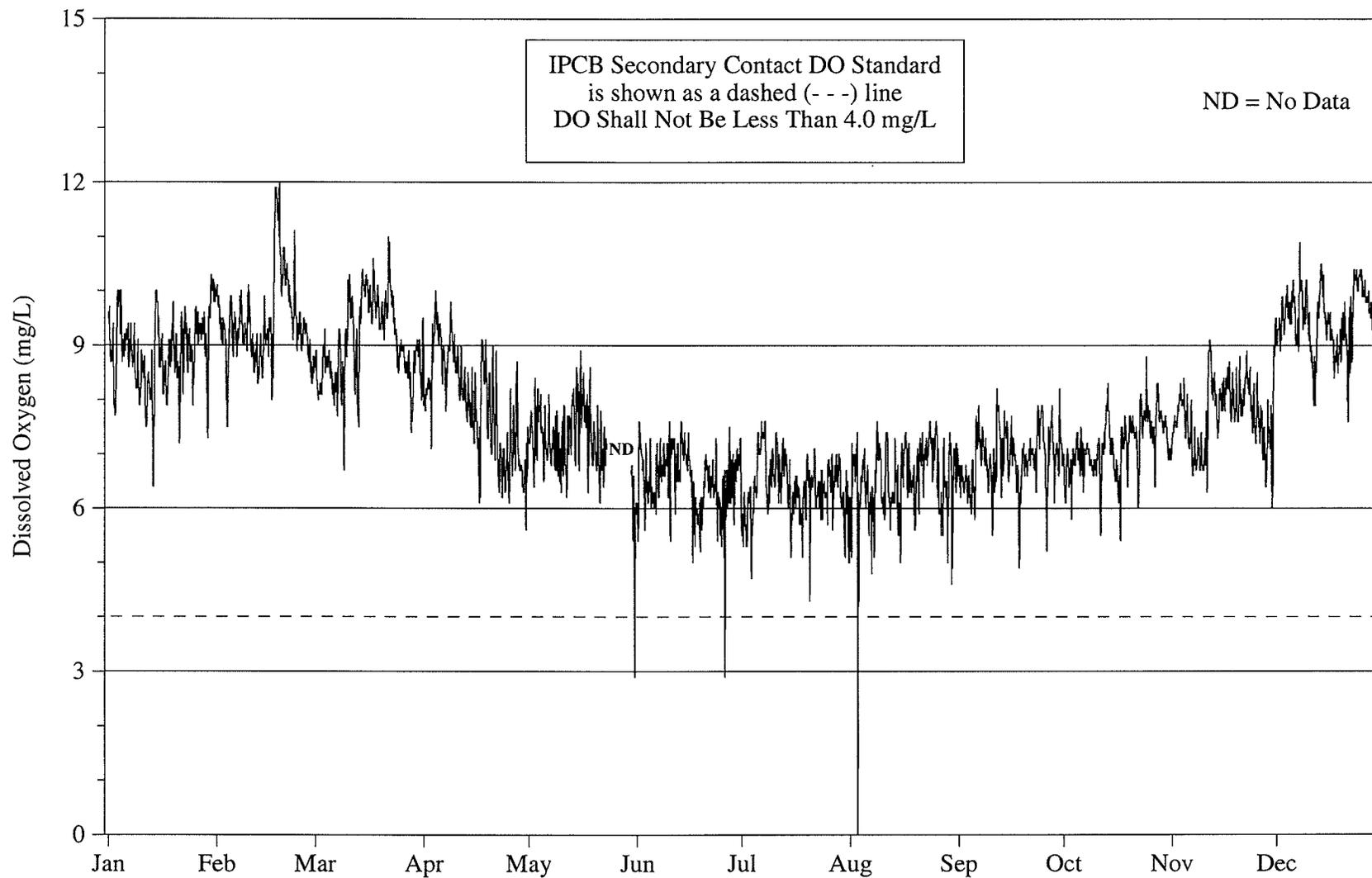
FIGURE 5: DISSOLVED OXYGEN CONCENTRATION MEASURED HOURLY AT FULLERTON AVENUE
