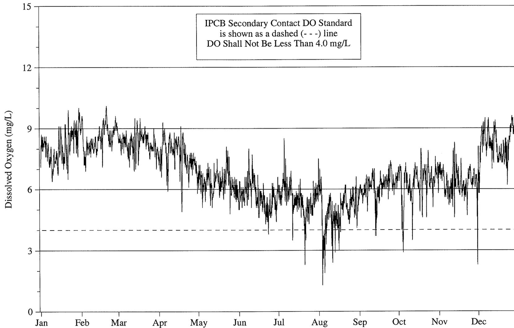
FIGURE 13: DISSOLVED OXYGEN CONCENTRATION MEASURED HOURLY AT ROUTE 83
