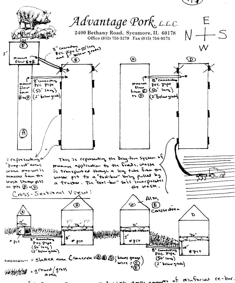
. = All "pits" are 4" thick-walled with ample amounts of reinforces re-bur.
