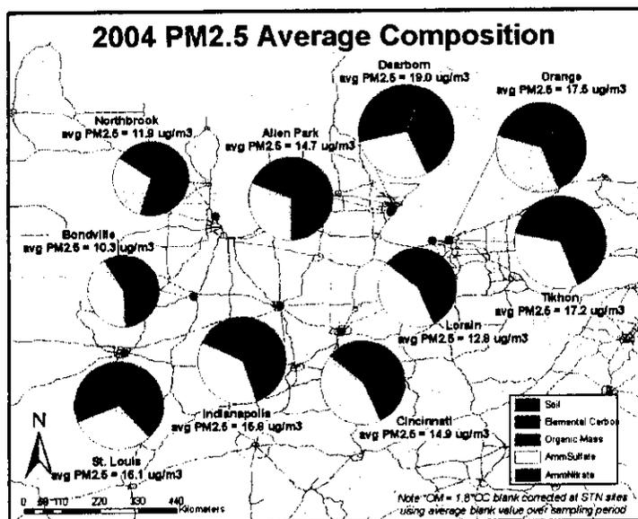
Figure 5. PM<sub>2.5</sub> chemical composition in the LADCO region – 2004 data
