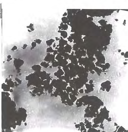
FIGURE NO. 12 Debris from dry brake compartment 5000x
