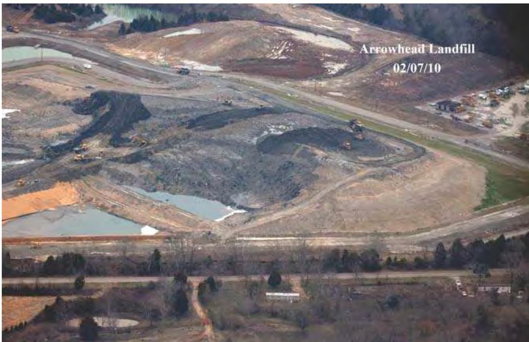
**Figure 10: Arrowhead Landfill, AL, disposal of TVA fly ash waste**
