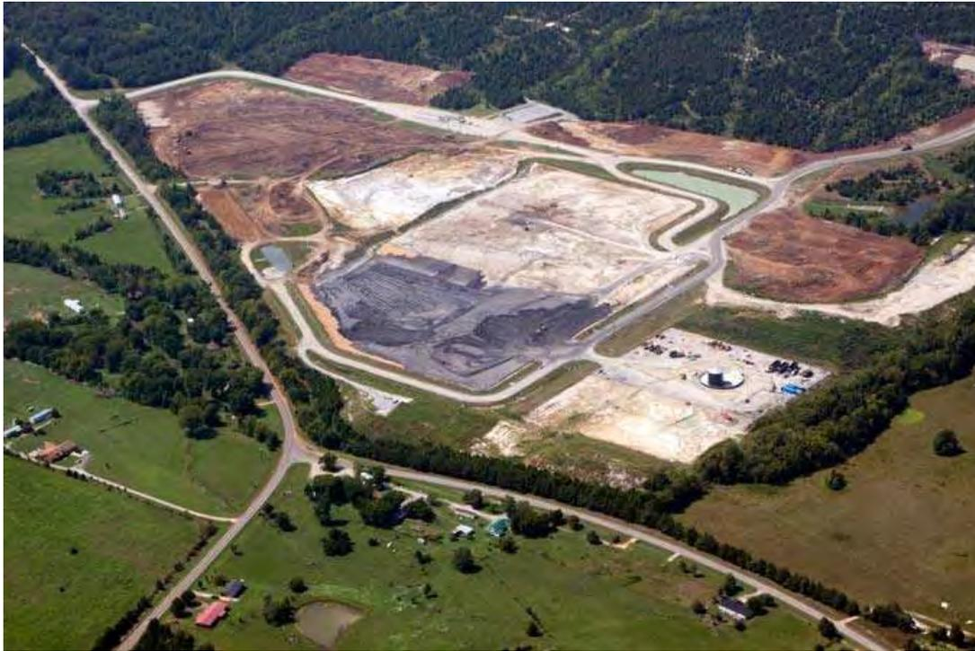
**Figure 9: Arrowhead Landfill, AL, disposal of fly ash from TVA Kingston pond spill**
