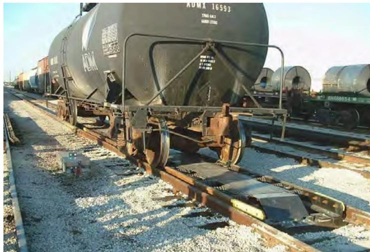
**Figure 4.** Inert retarder is engaged.
