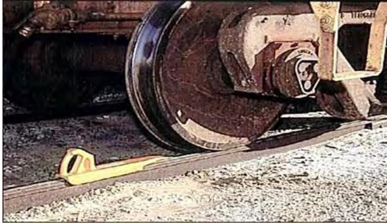
**Figure 3.** Skate is not engaged. Noncompliant for securement.
