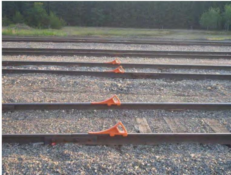
**Figure 2.** Skates at clearance points. Noncompliant for securement.
