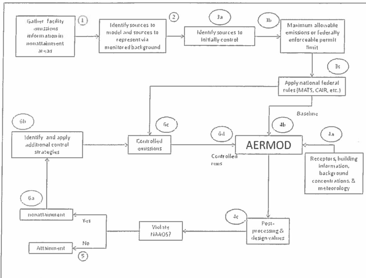
Figure 2. Flowchart of SO<sub>2</sub> Modeling Framework for SIP Demonstration.
