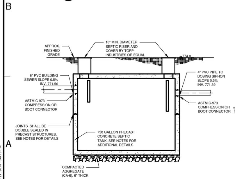
**A1 SEPTIC TANK ELEVATION**
