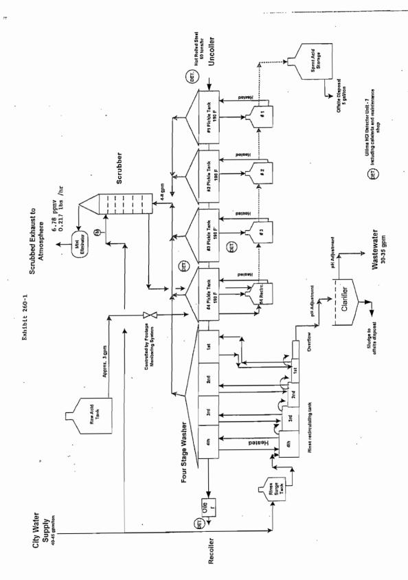
NACME Pickling Process Flow Diagram
