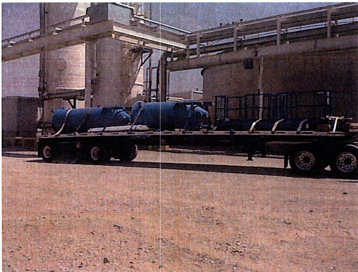
Figure 8 Parkson D2 Sand Filters (Foreground on trailer)
