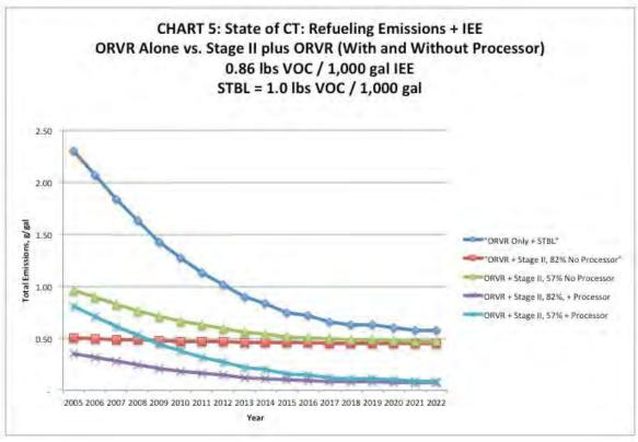
As seen in Chart 5, the ORVR + Stage II + Processor curves show a large reduction in total emissions from the ORVR Alone case, when STBL emissions are properly accounted for in the emissions inventory. We use a very conservative figure of 1.0 lbs. VOC / 1,000 gal for STBL; in practice ARID has measured values nearly five times higher than this figure, or about 5 lbs. of VOC per 1,000 gallons of fuel dispensed.
