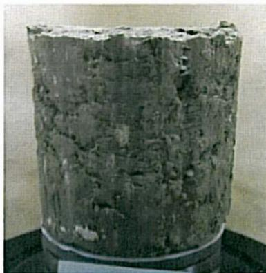
Note: A B-value of 0.96 was achieved for the undisturbed specimen. Permeation measurements were made with a mercury U-tube. The effective confining pressure was 5 psi per test request.
