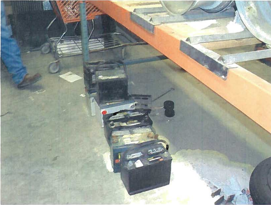
Date: 10/25/2011 Time: 11:36 A.M. Direction: northeast Photo by: S. Williams Exposure #: 001 Comments: apparent fluid has leaked from at least one of the batteries
