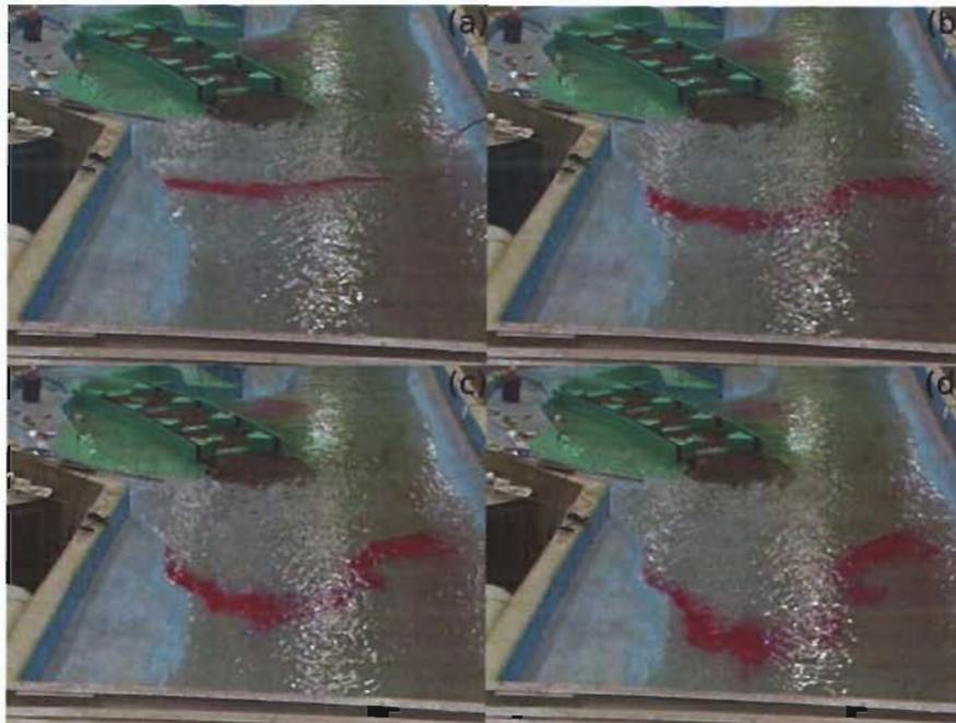
**Figure 7.13 – Evolution of dye injected downstream of the canoe chute at cross-section G.**
