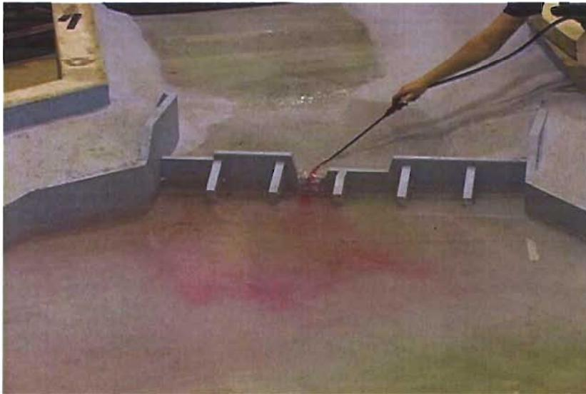
**Figure 5.13 – Dye injection upstream of the spillway for the 85% exceedance discharge.**
