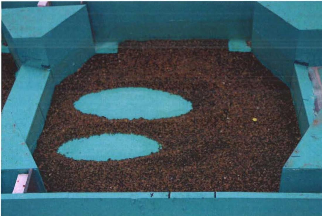
**Figure 7.15 – Photograph of erosional depressions observed in pool 3 after running the 5% exceedance discharge.**
