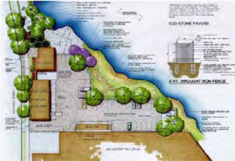
Figure 6.7 Example of riverfront industrial site utilizing riverbank recontouring, infiltration area, and porous pavers for stormwater management.
