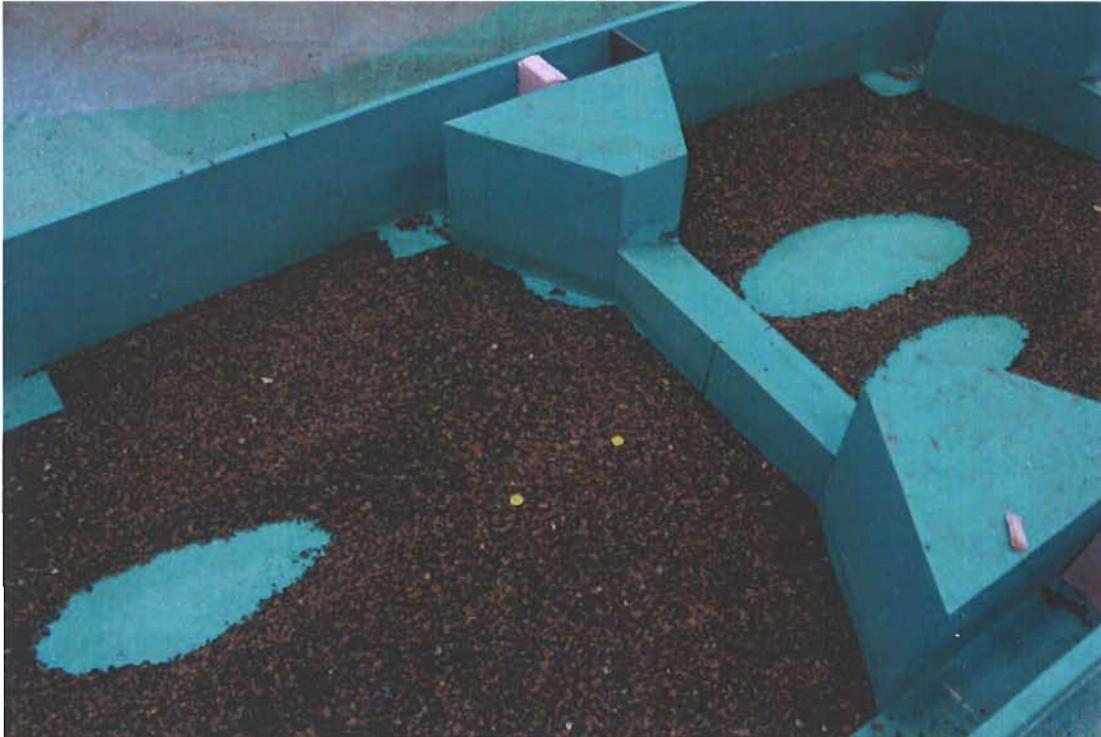
**Figure 7.16 – Erosion observed at the upstream face of drop 3 after running the 5% exceedance discharge.**
