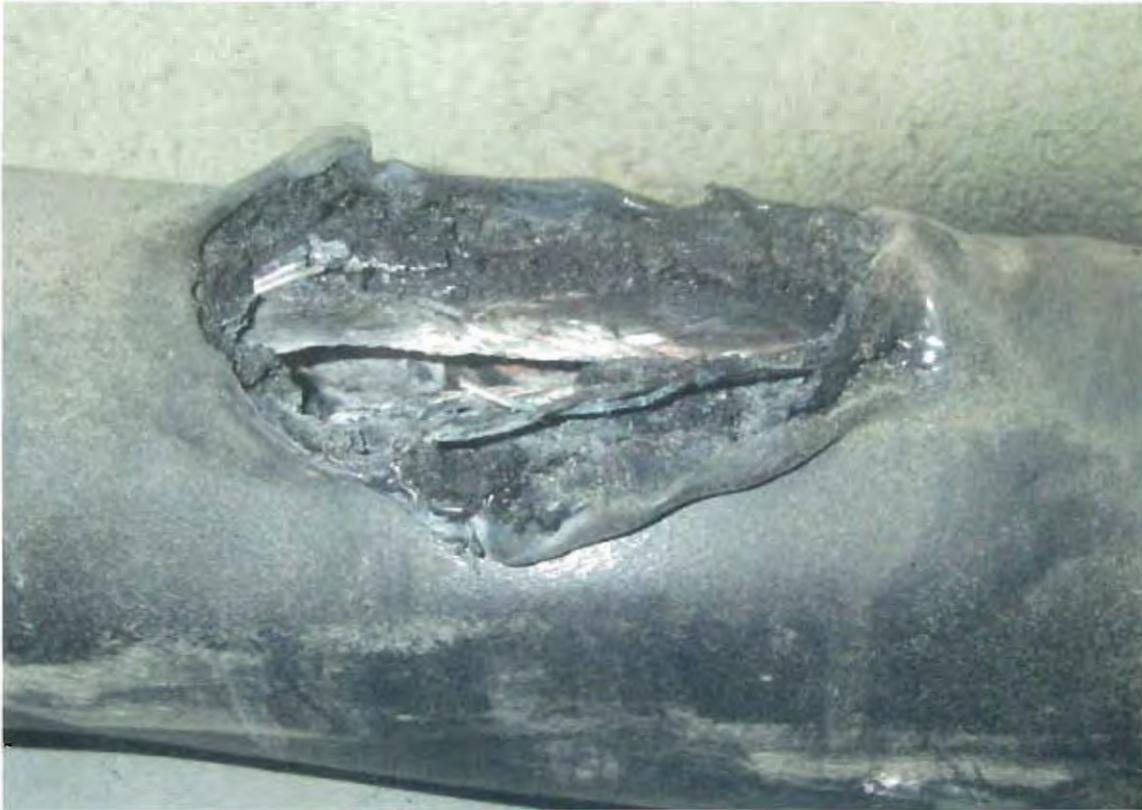
2. Umbilical Failure (Teflon tubes that carry mercury sample melted from heat trace over heating)
