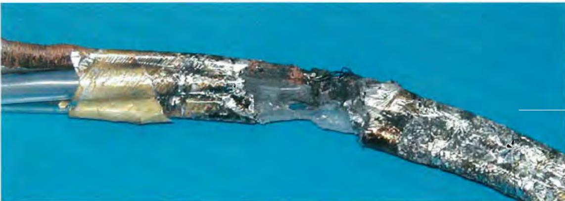
3. Umbilical Failure (Teflon tubes that carry mercury sample begin to melt)
