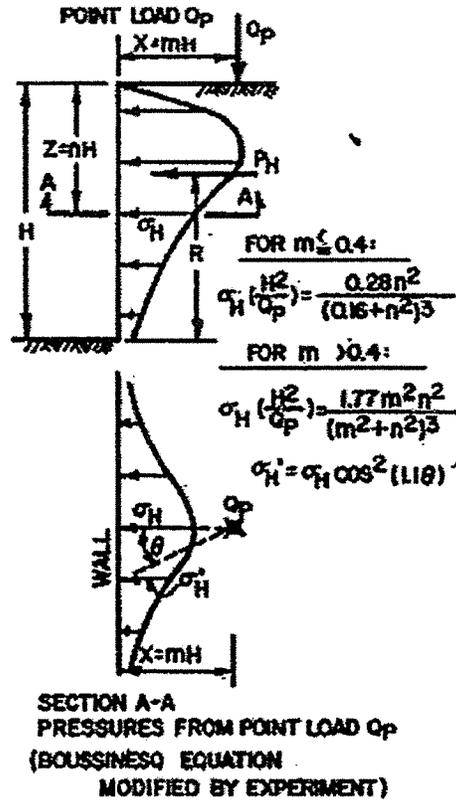
PRESSURE ON FOUNDATION WALL DUE TO A SURFACE POINT LOAD
