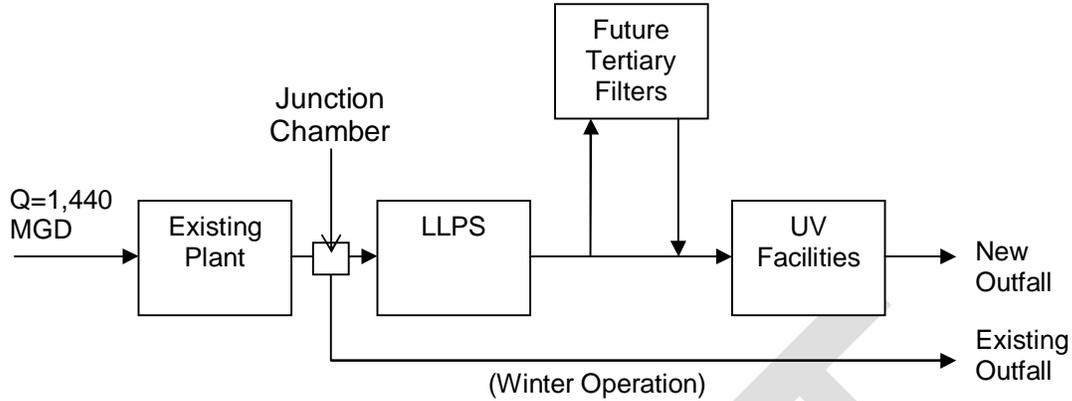
**Figure ES 1 - Proposed UV Facilities Flow Diagram**
