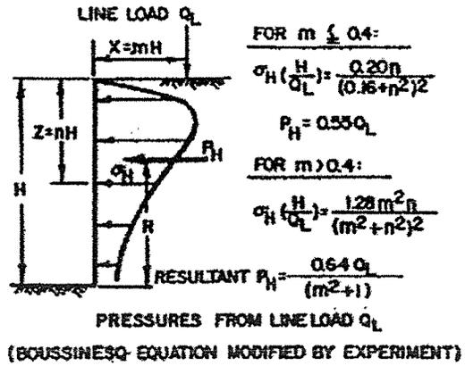
PRESSURE ON FOUNDATION WALL DUE TO A SURFACE LINE LOAD
