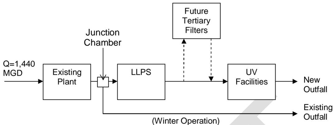
**Figure 3.3-1 - Proposed UV Disinfection Flow Diagram**
