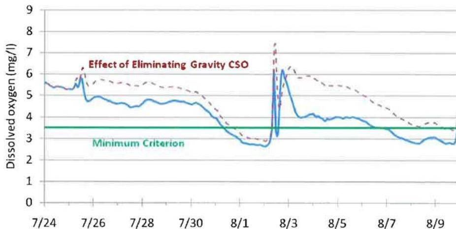
**Figure 5. Comparison of Dissolved Oxygen Levels at Halsted Street, SBCR for Existing Conditions and Elimination of Gravity CSOs (2001)**
