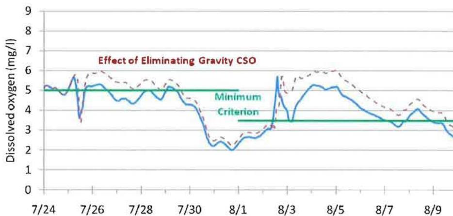
**Figure 4. Comparison of Dissolved Oxygen Levels at Kinzie Street, NBCR for Existing Conditions and Elimination of Gravity CSOs (2001)**
