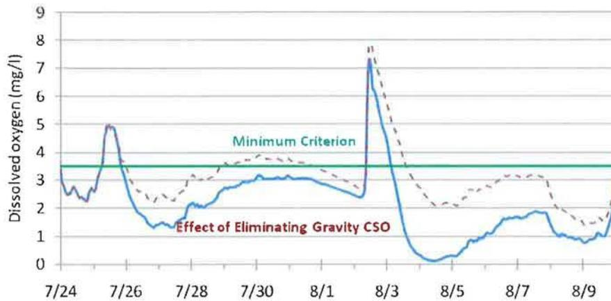
**Figure 6. Comparison of Dissolved Oxygen Levels at B&O Railroad Bridge, CSSC for Existing Conditions and Elimination of Gravity CSOs (2001)**
