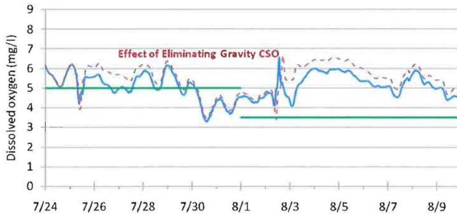
**Figure 3. Comparison of Dissolved Oxygen Levels at Fullerton Avenue, NBCR for Existing Conditions and Elimination of Gravity CSOs (2001)**
