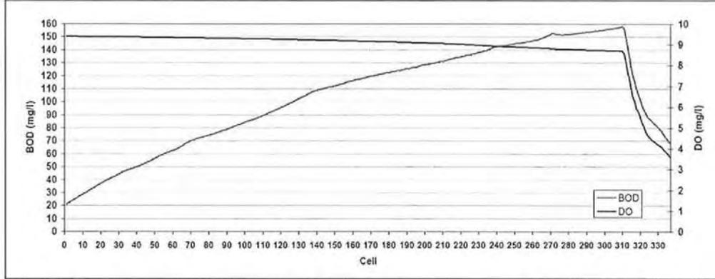
FIG. 31. BOD and DO longitudinal concentration profiles in Bubbly Creek after the CSO discharge.
