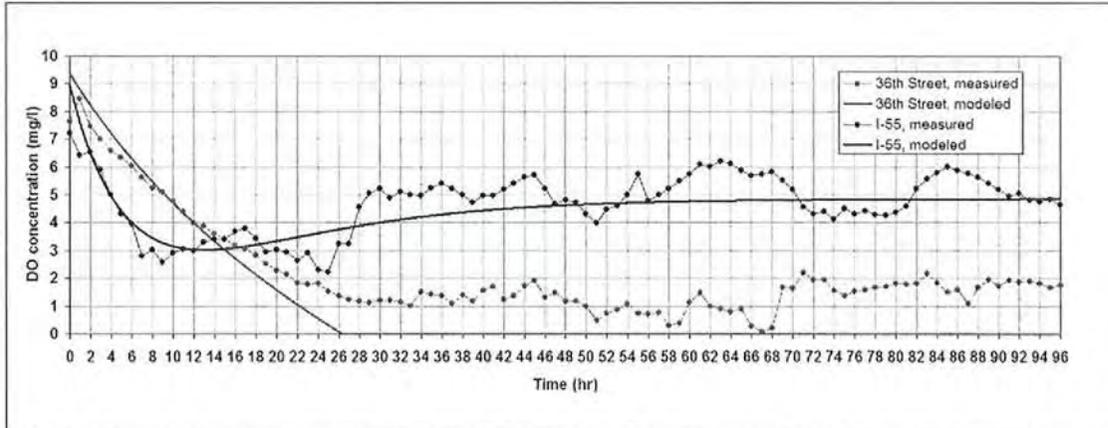
**FIG. 34. DO concentration evolution at the two monitoring stations in Bubbly Creek. Measured and modeled values.**
