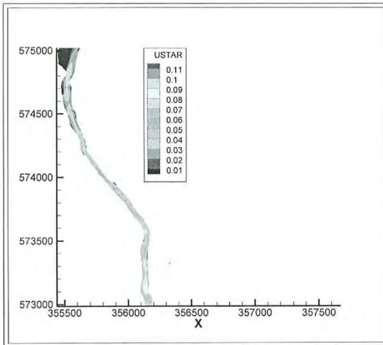
FIG. 26. Shear velocity field (m/s) for a discharge of  $69.43 \text{ m}^3/\text{s}$ .
