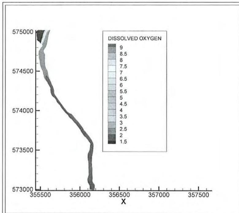
FIG. 30. Concentration of DO (mg/l) in the water column, for a flow discharge of 69.43 m<sup>3</sup>/s, after 7.66 hours.
