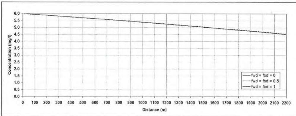
**FIG. 11. Sensitivity analysis of the model to the dissolved fractions of BOD in the water column and in the bed: longitudinal profiles of the concentration of DO in the water column after 10 hours.**
