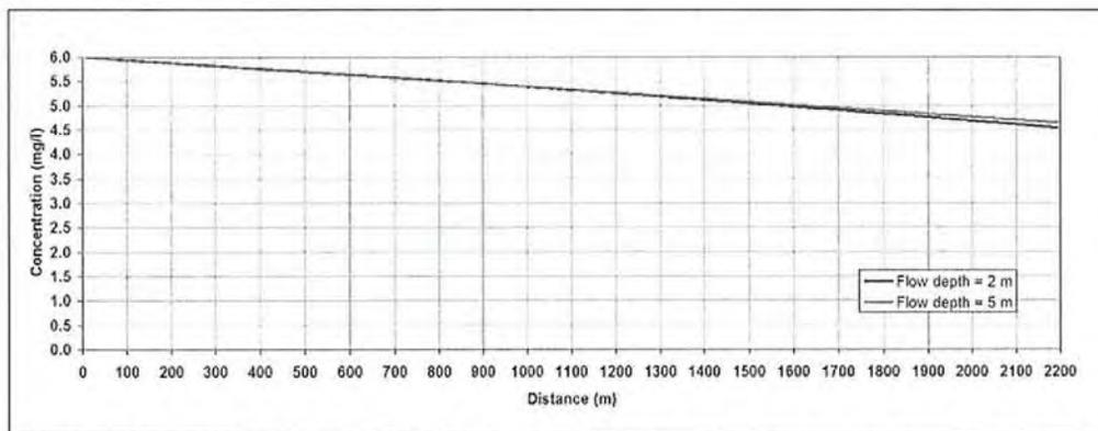
**FIG. 9. Sensitivity analysis of the model to the flow depth: longitudinal profiles of the concentration of DO in the water column after 10 hours.**
