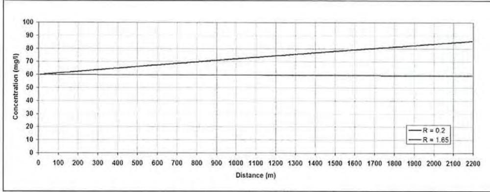
FIG. 16. Sensitivity analysis of the model to the submerged specific gravity of solids: longitudinal profiles of the concentration of BOD in the water column after 10 hours.
