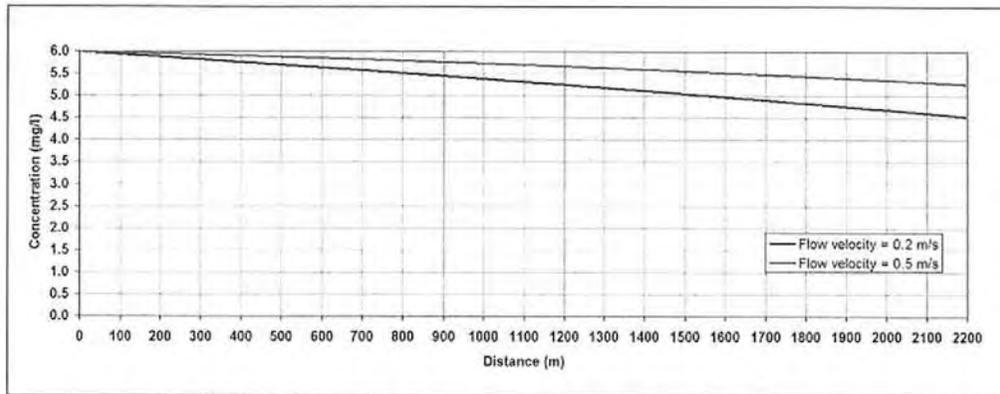
**FIG. 7. Sensitivity analysis of the model to the flow velocity: longitudinal profiles of the concentration of DO in the water column after 10 hours.**
