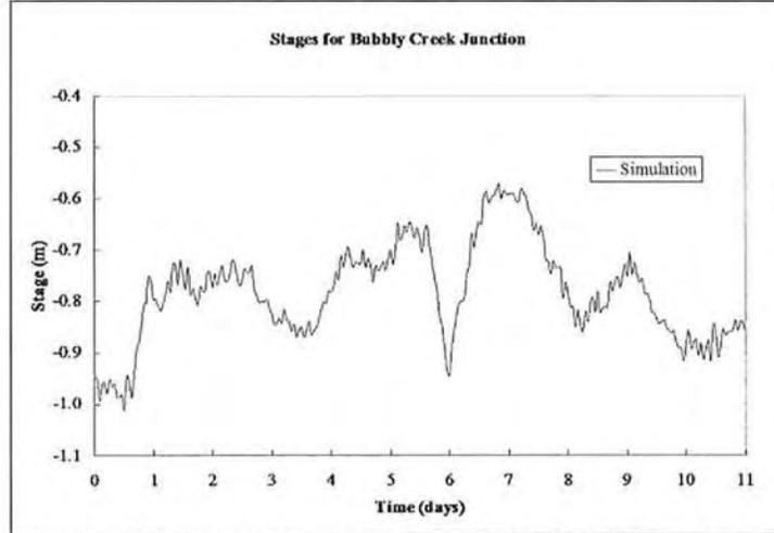
FIG. 32. Typical water stage oscillation at Bubbly Creek’s mouth (results from hydrodynamic 3-D modeling).
