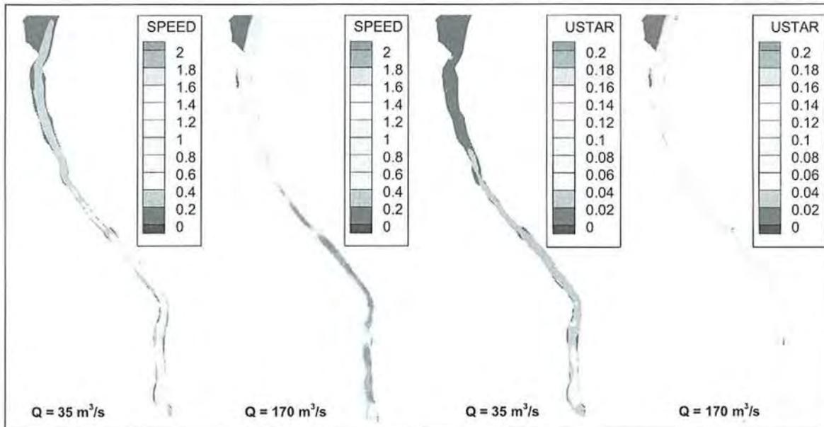
Figure 5. Comparison between the velocity (“SPEED” in m/s) and shear velocity (“USTAR” in m/s) fields in the creek for discharges of  $35 \text{ m}^3/\text{s}$  and  $170 \text{ m}^3/\text{s}$ , respectively.
