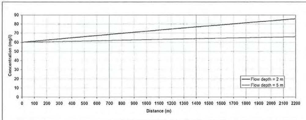
**FIG. 8. Sensitivity analysis of the model to the flow depth: longitudinal profiles of the concentration of BOD in the water column after 10 hours.**
