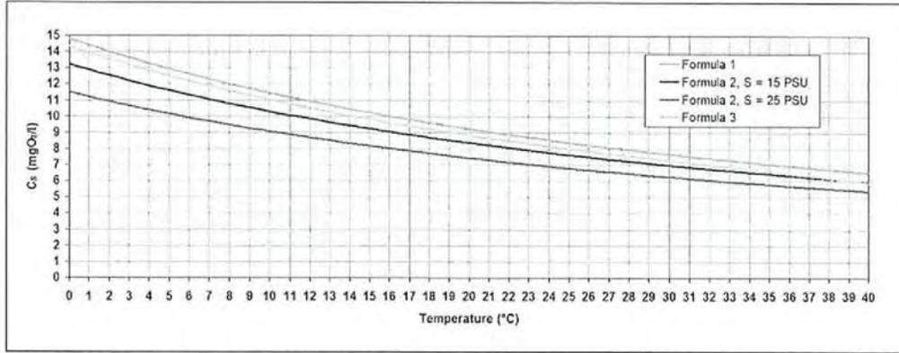
FIG. 1. Comparison between the different formulae for the calculation of the dissolved oxygen concentration at saturation  $C_S$ .
