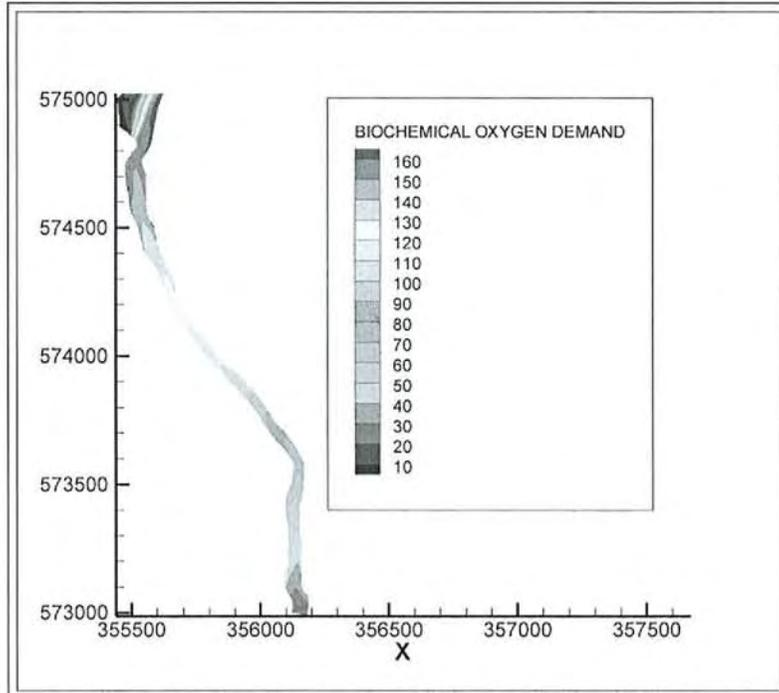
FIG. 29. Concentration of BOD (mg/l) in the water column, for a flow discharge of 69.43 m<sup>3</sup>/s, after 7.66 hours.
