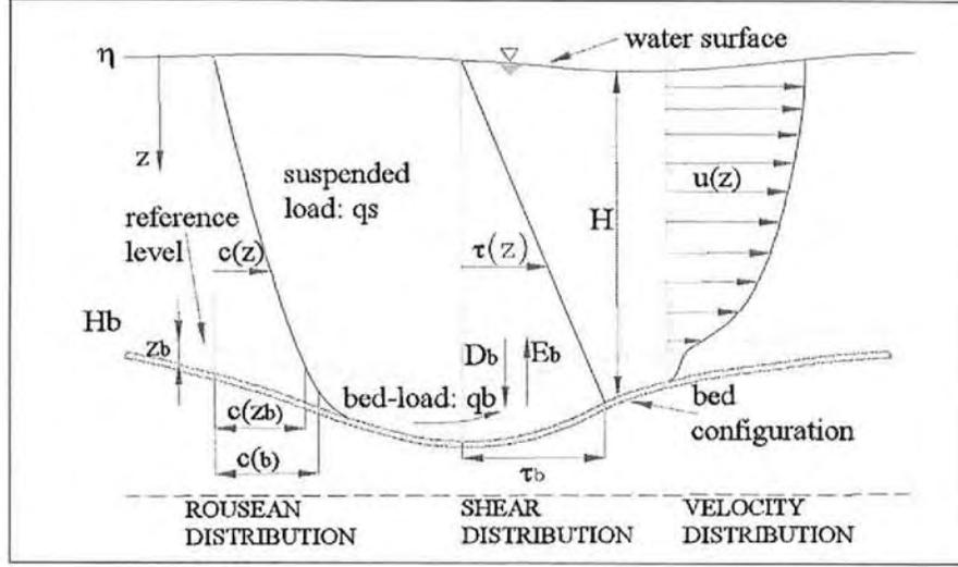
FIG. 2. Sediment model configuration.
