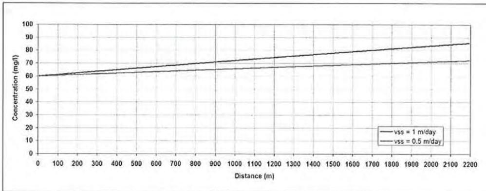
**FIG. 14. Sensitivity analysis of the model to the settling velocity of solids: longitudinal profiles of the concentration of BOD in the water column after 10 hours.**
