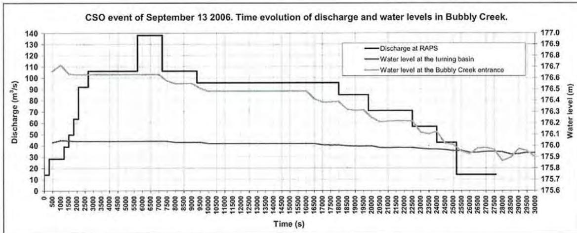
Figure 4. Evolution of discharge and water levels at the Bubbly Creek upstream and downstream ends for the CSO event of September 13 2006.
