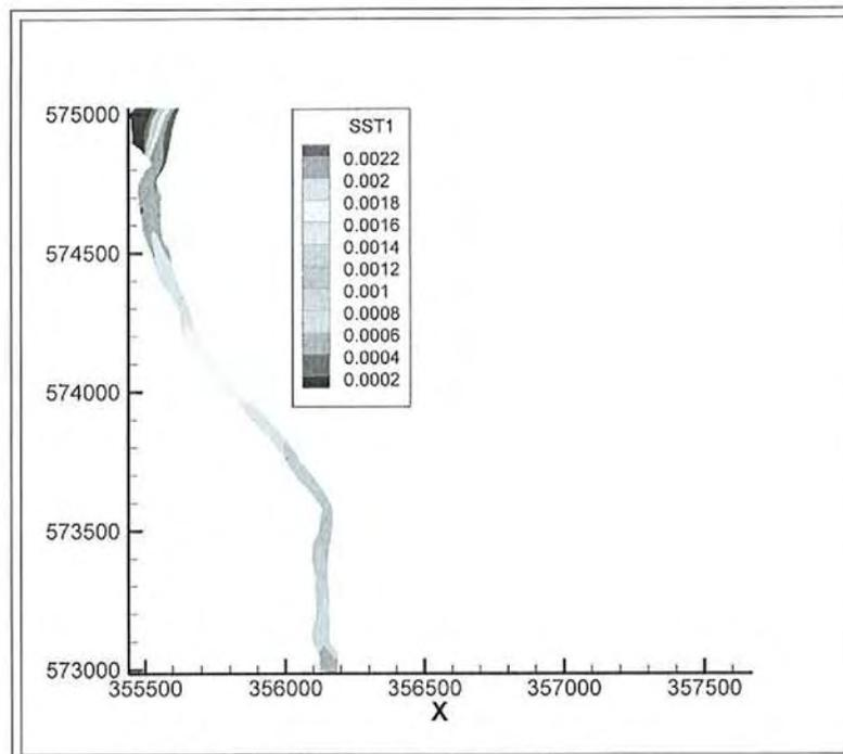
FIG. 28. Volume concentration of suspended solids in the water column, for a flow discharge of  $69.43 \text{ m}^3/\text{s}$ , after 7.66 hours.
