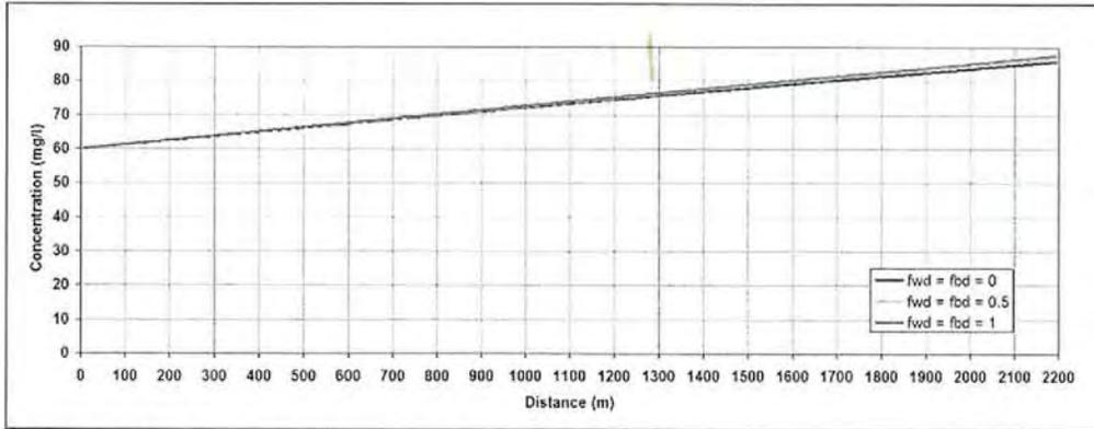
**FIG. 10. Sensitivity analysis of the model to the dissolved fractions of BOD in the water column and in the bed: longitudinal profiles of the concentration of BOD in the water column after 10 hours.**
