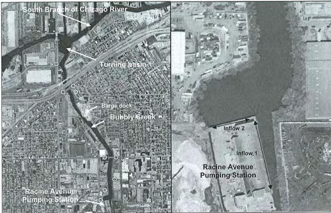
Figure 1. Aerial view of Bubbly Creek with the location of the CSO outfalls along the creek (circles) and detail of the Racine Avenue Pumping Station (RAPS) with the location of “Inflow 1” and “Inflow 2”.
