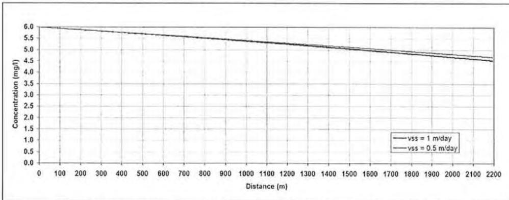
**FIG. 15. Sensitivity analysis of the model to the settling velocity of solids: longitudinal profiles of the concentration of DO in the water column after 10 hours.**
