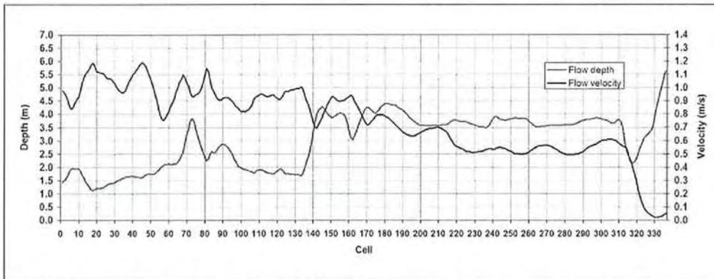
FIG. 25. Longitudinal profiles of flow depth and velocity along the centerline of Bubbly Creek.
