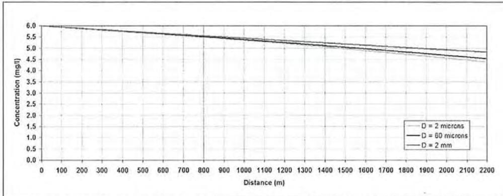
**FIG. 13. Sensitivity analysis of the model to the effective diameter of solids: longitudinal profiles of the concentration of DO in the water column after 10 hours.**
