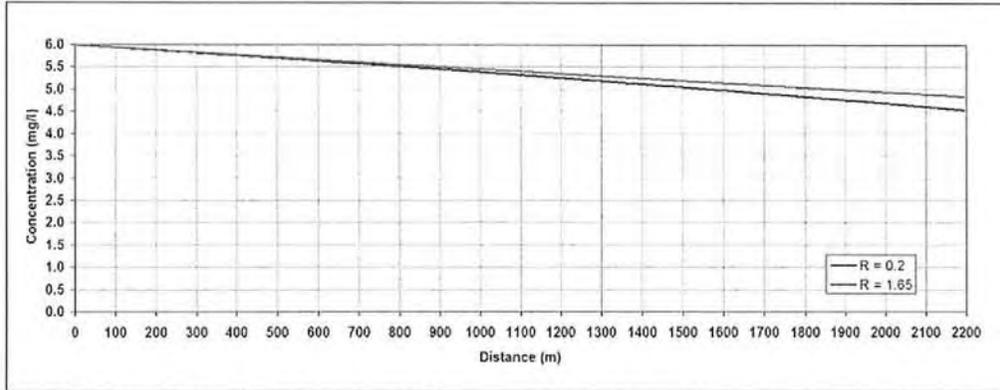
FIG. 17. Sensitivity analysis of the model to the submerged specific gravity of solids: longitudinal profiles of the concentration of DO in the water column after 10 hours.
