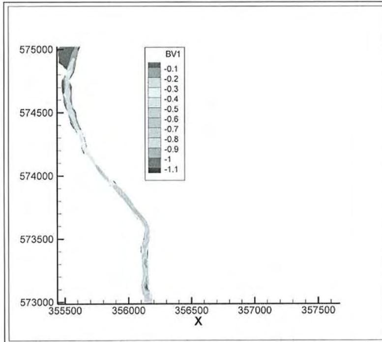
FIG. 27. Cumulated bed elevation variation (m), for a flow discharge of  $69.43 \text{ m}^3/\text{s}$ , after 7.66 hours.
