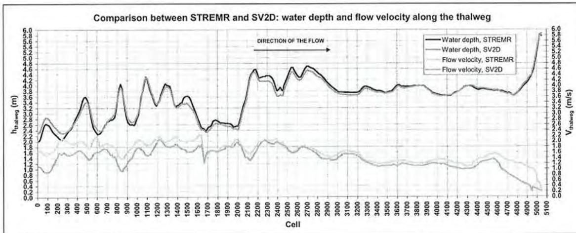
Figure 2. Comparison between the water depths and the flow velocities calculated along the thalweg of the creek by STREMR and SV2D.
