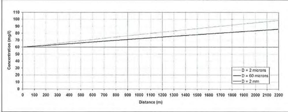
**FIG. 12. Sensitivity analysis of the model to the effective diameter of solids: longitudinal profiles of the concentration of BOD in the water column after 10 hours.**
