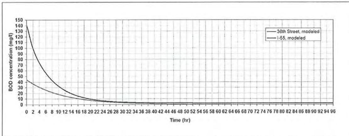
FIG. 33. BOD concentration evolution at the two monitoring stations in Bubbly Creek. Modeled values.
