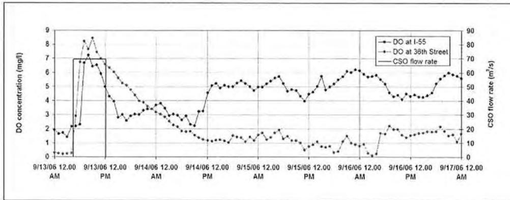
**FIG. 21. Dissolved oxygen at 36<sup>th</sup> Street and I-55 monitoring stations during and after the CSO event on September 13 2006.**
