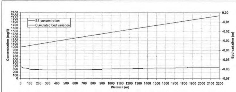
**FIG. 3. Longitudinal profile of the concentration of suspended solids in the water column and of the cumulated bed variation after 10 hours.**
