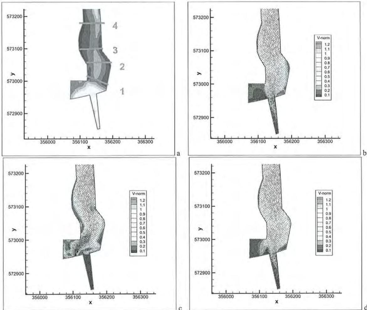
**Figure 3. Results of the sensitivity analysis on the influence of the location of the combined-sewer-overflow discharge input in terms of flow velocity. (a) Sections considered for the analysis, (b) CSO from the 9 pumps along "Inflow 1", (c) CSO from the 5 pumps along "Inflow 2", and (d) CSO distributed over "Inflow 1" and "Inflow 2".**
