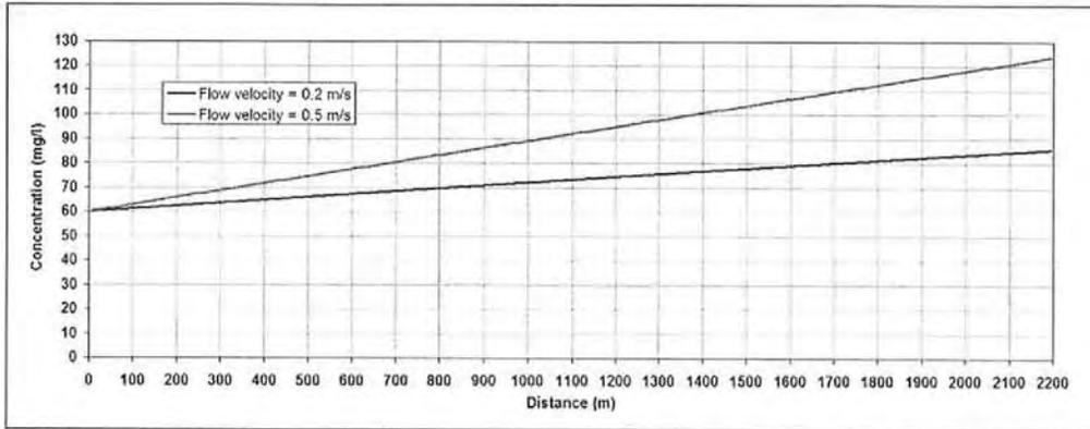
**FIG. 6. Sensitivity analysis of the model to the flow velocity: longitudinal profiles of the concentration of BOD in the water column after 10 hours.**
