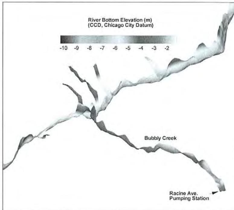
**FIG. 19. Typical bathymetry of Bubbly Creek and the South Branch of the Chicago River. The reference is the Chicago City datum (CCD) at 176.63 m above sea level.**
