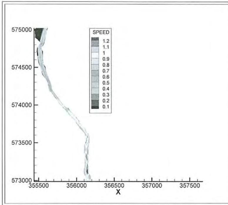
FIG. 24. Flow velocity field (m/s) for a discharge of  $69.43 \text{ m}^3/\text{s}$ .
