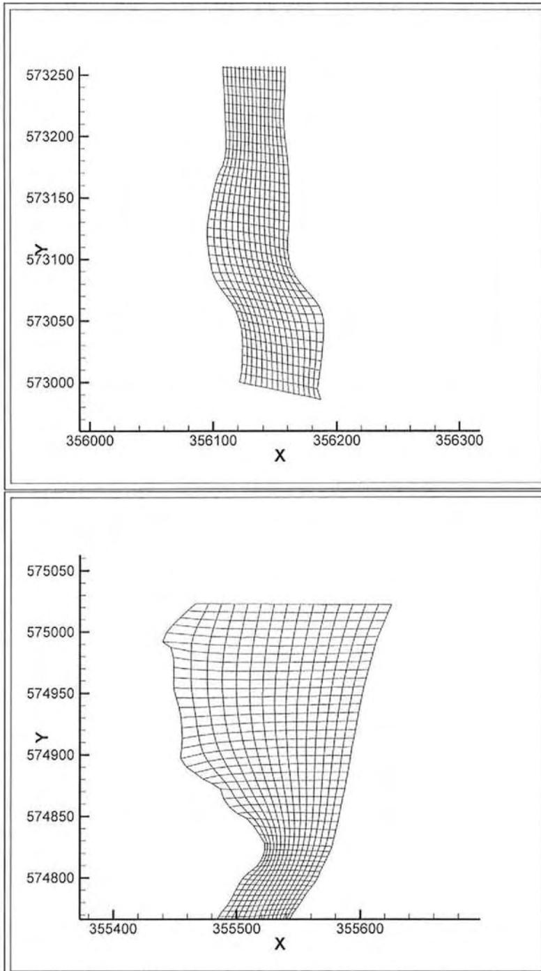
FIG. 22. Details of the computational mesh for Bubbly Creek (upstream and downstream ends).
