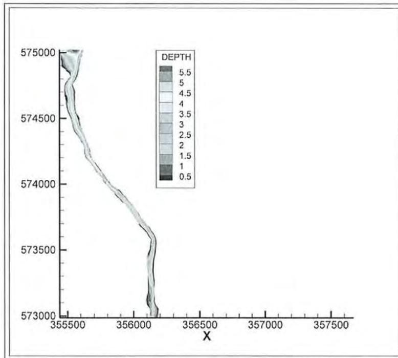
FIG. 23. Water depth field (m) in Bubbly Creek.
