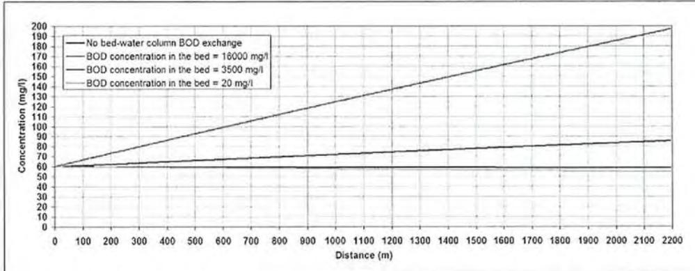
**FIG. 4. Sensitivity analysis of the model to the BOD concentration in the bed: longitudinal profiles of the concentration of BOD in the water column after 10 hours.**
