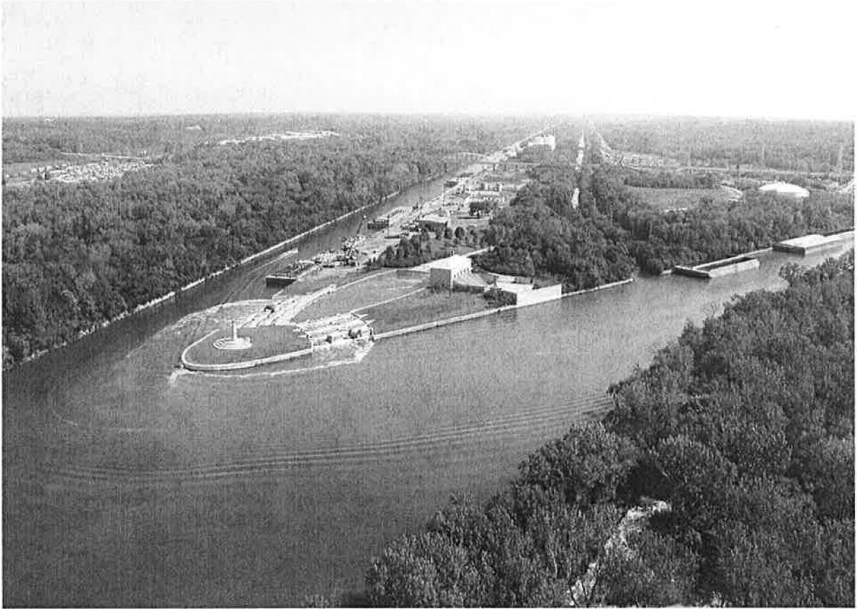
Attachment 1, Looking north at junction of the Calumet-Sag Channel (right foreground) with the Chicago Sanitary and Ship Canal (left background). Opening to Illinois and Michigan Canal visible to the left of the first barge on the Calumet-Sag Channel).
