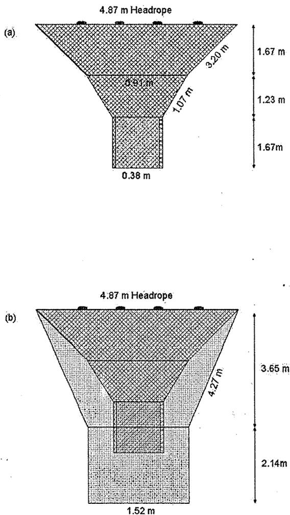
FIGURE 2.—Trawl designs for (a) a standard two-seam balloon trawl (used to sample the upper Mississippi River in 1991–1997) and (b) a modified (Missouri) trawl (used for sampling in 1998–2001).
