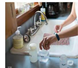
Water quality testing including first draw and 3 minute flush is required to determine influence of corrosion on presence of heavy metals in drinking water.
