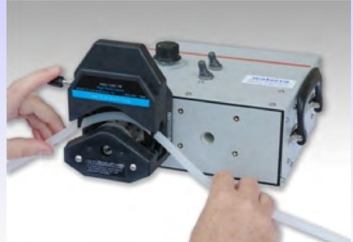
**Battery-powered peristaltic pump**
