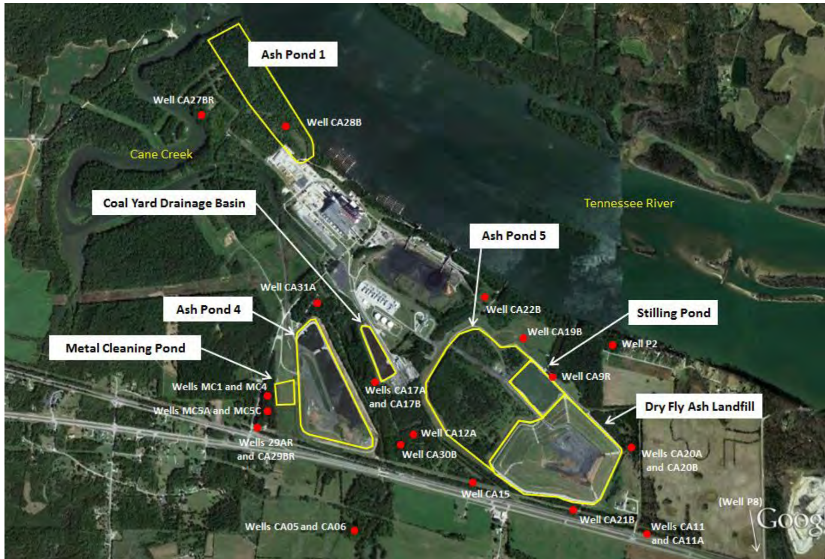
Figure 4-1: Groundwater wells at Colbert Fossil Plant (approximate locations)
