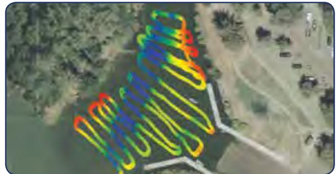
Bathymetric Image using single beam Echosounder Image
