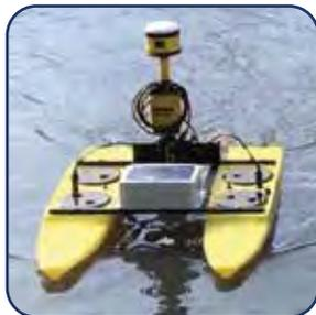
HydroLite-TM mounted on HyDrone-ASV
