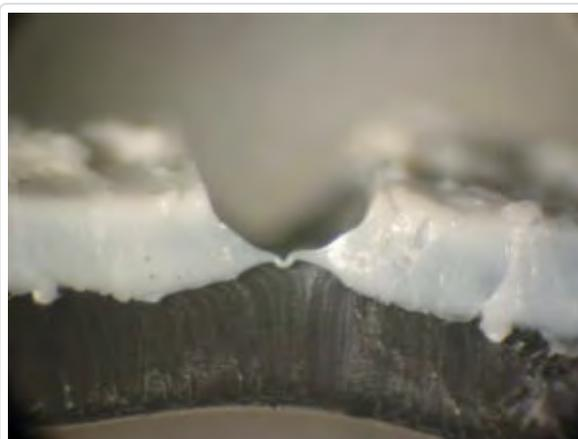
*FIGURE 5 Photograph from 2014 of original razor-blade slit that extended through the white surface into the VLDPE core. During the NCTL stress-crack test, the sharp notch eventually blunted and did not propagate, which is a testimony to the functionality of the VLDPE core to resist stress cracking. No photographs were taken in 2018, but the NCTL results indicated continued very strong performance for this test.*
