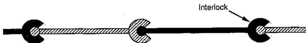
Figure 7.5 - Interlocking Steel Sheet Piles.
