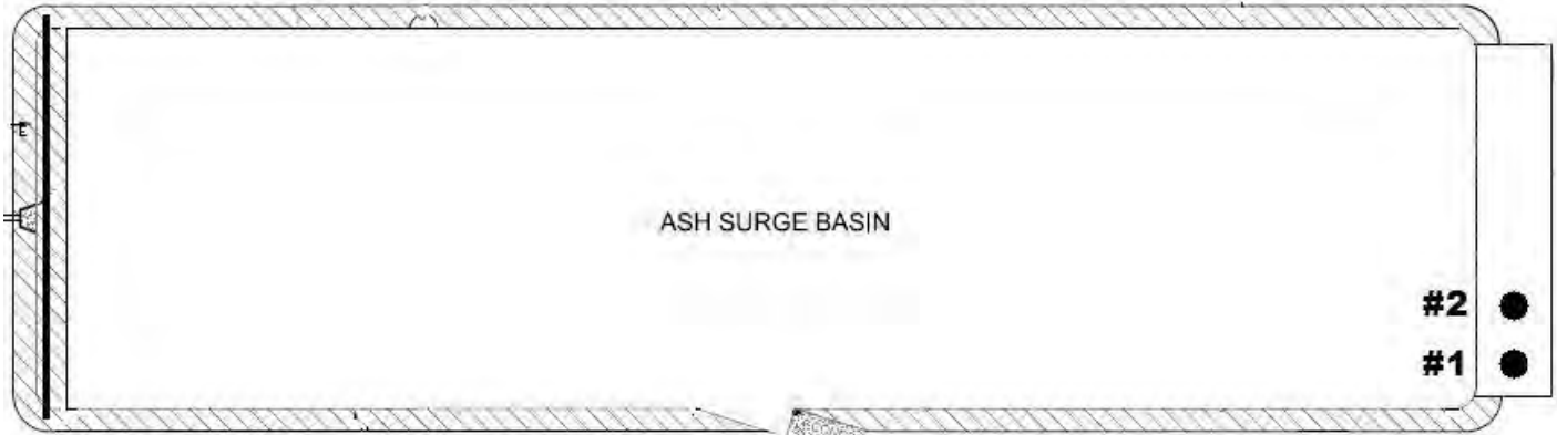
FIGURE 1. APPROXIMATE LOCATIONS OF THE LEAKS FOUND IN THE ASH SURGE BASIN
